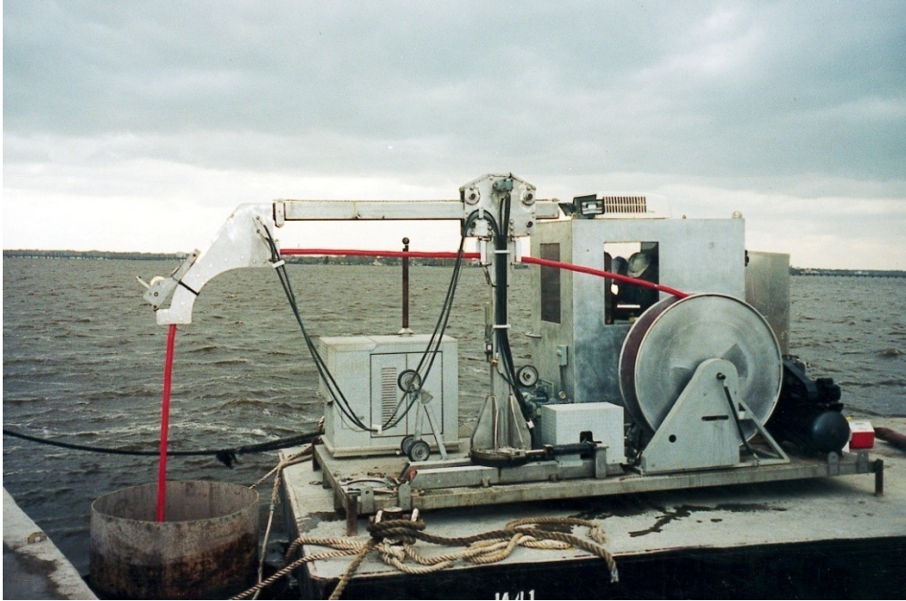
Figure 40, Shaft Inspection Device
