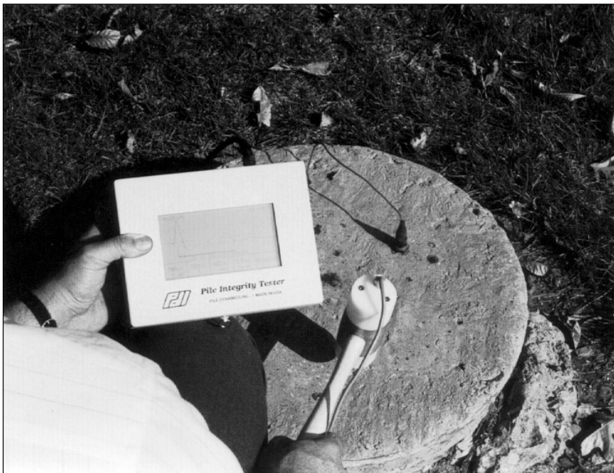
Figure 39, Pile Integrity Tester (After PDI, 1993)
