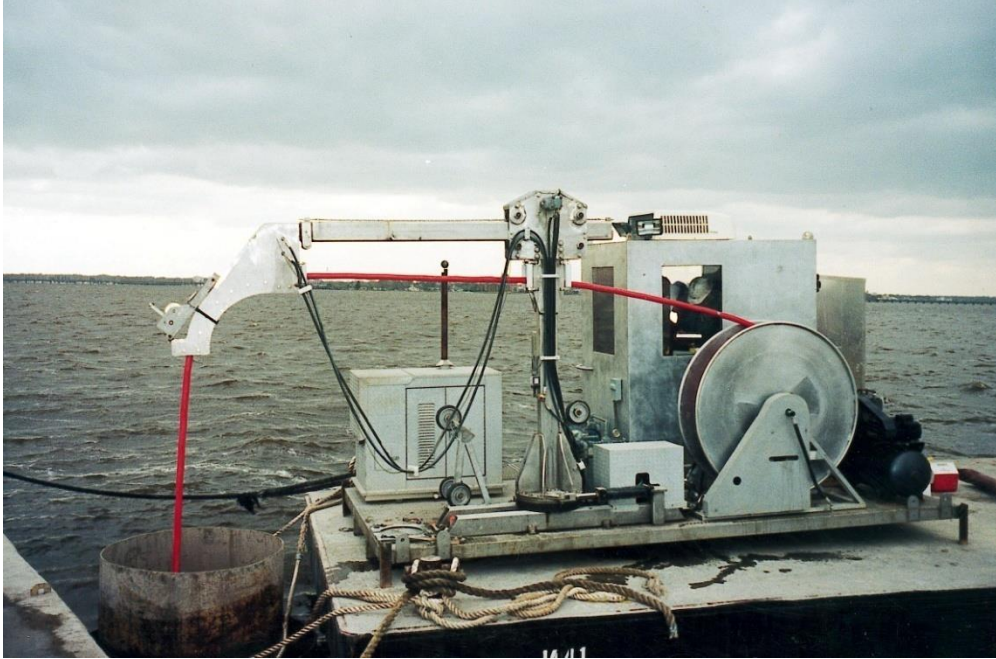
Figure 41, Shaft Inspection Device
