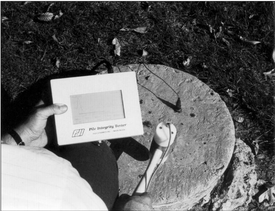
Figure 40, Pile Integrity Tester (After PDI, 1993)
