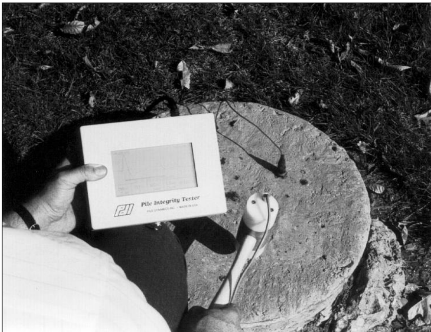
Figure 40, Pile Integrity Tester (After PDI, 1993)
