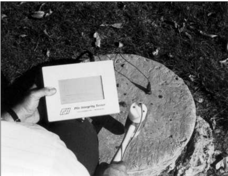
Figure 42, Pile Integrity Tester (After PDI, 1993)
