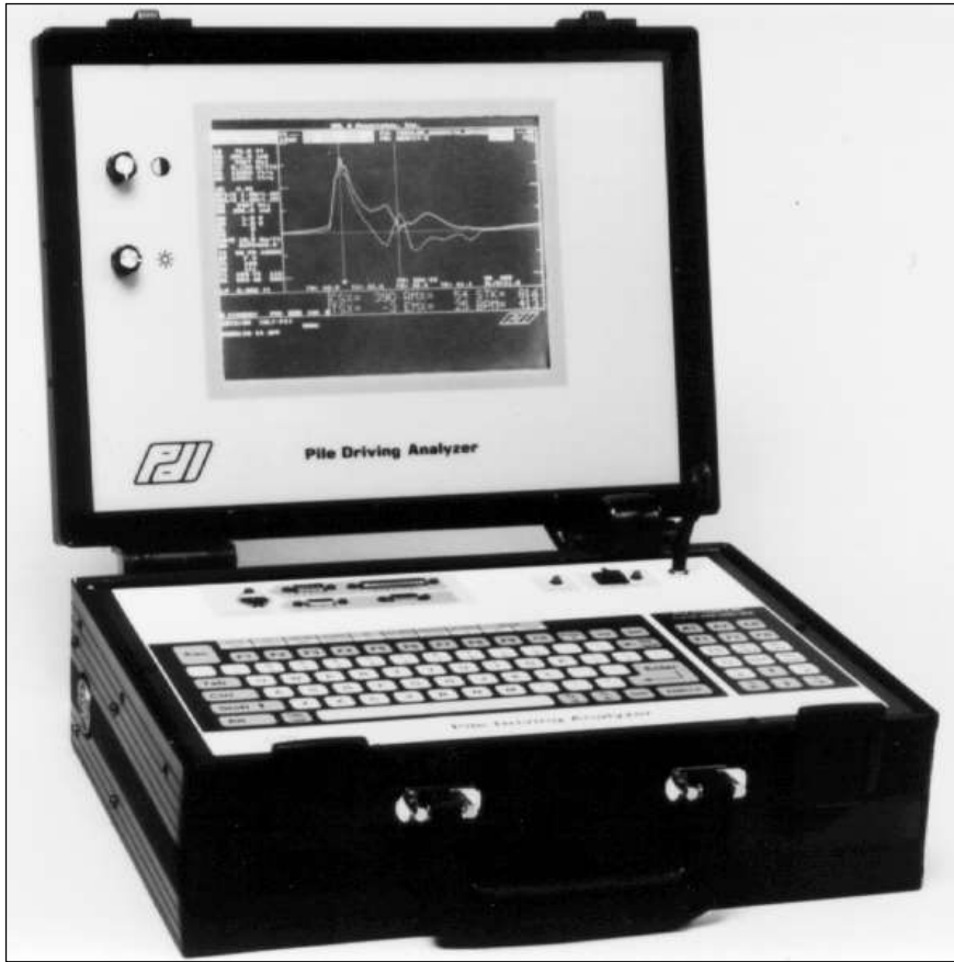
Figure 37, Pile Driving Analyzer, Model PAK (After PDI, 1993)
