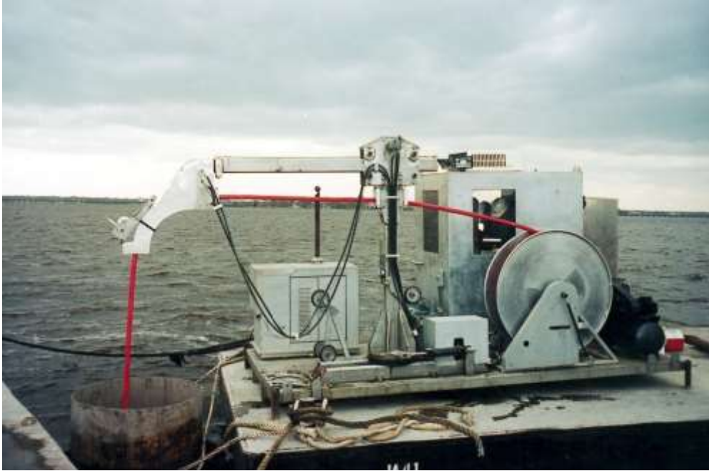
Figure 43, Shaft Inspection Device
