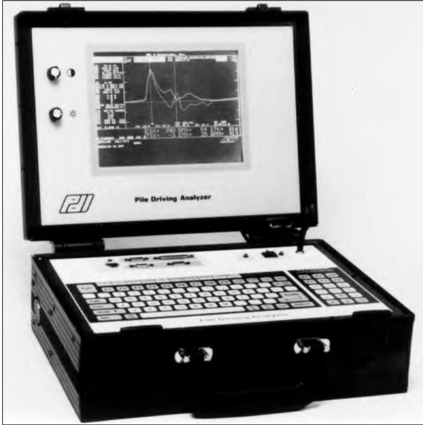
Figure 37, Pile Driving Analyzer, Model PAK (After PDI, 1993)
