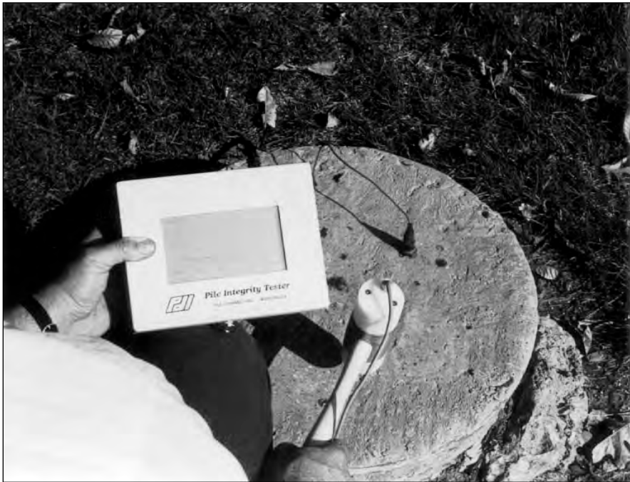
Figure 42, Pile Integrity Tester (After PDI, 1993)
