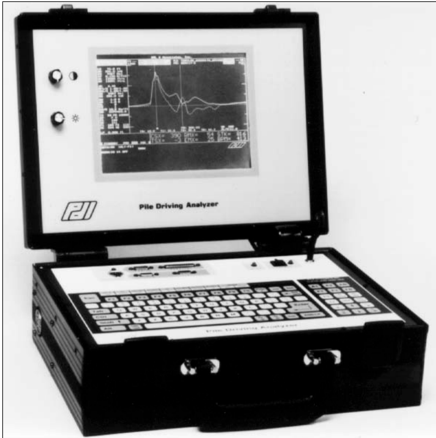
Figure 37, Pile Driving Analyzer, Model PAK (After PDI, 1993)
