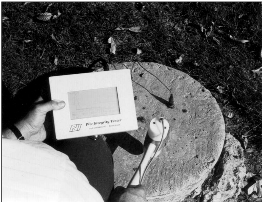
Figure 42, Pile Integrity Tester (After PDI, 1993)
