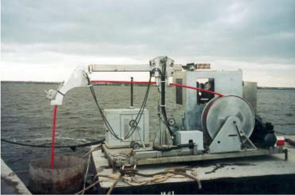
**Figure 39, Shaft Inspection Device**
