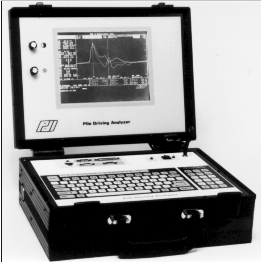
**Figure 33, Pile Driving Analyzer, Model PAK (After PDI, 1993)**
