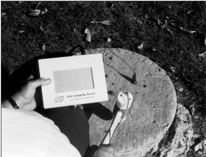
**Figure 34, Pile Integrity Tester (After PDI, 1993)**
