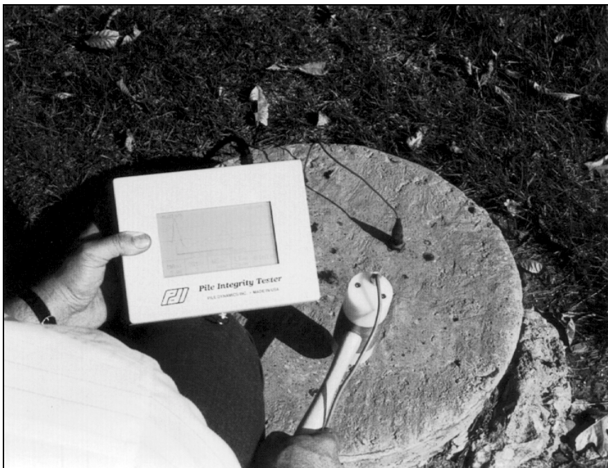
Figure 34, Pile Integrity Tester (After PDI, 1993)
