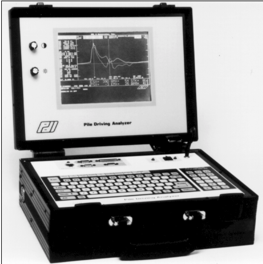
Figure 33, Pile Driving Analyzer, Model PAK (After PDI, 1993)
