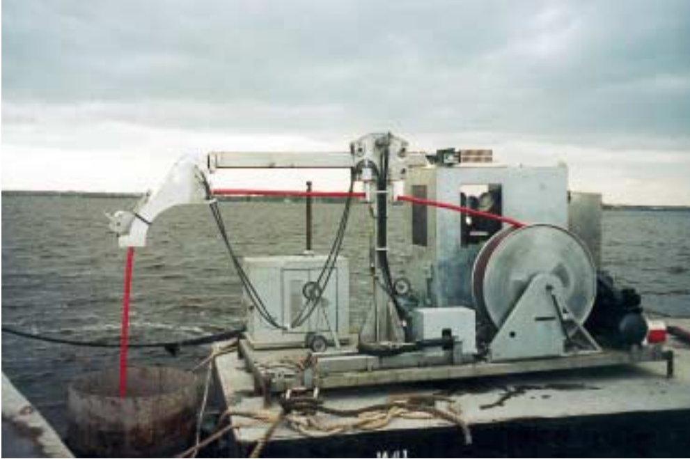
Figure 39, Shaft Inspection Device
