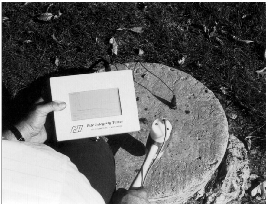
Figure 39, Pile Integrity Tester (After PDI, 1993)
