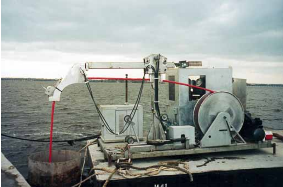
Figure 43, Shaft Inspection Device
