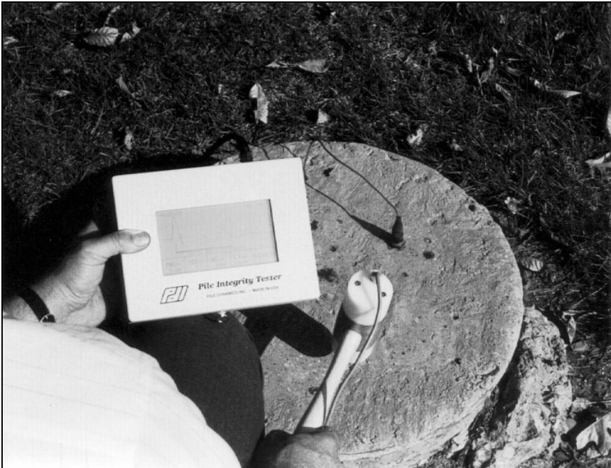
Figure 42, Pile Integrity Tester (After PDI, 1993)
