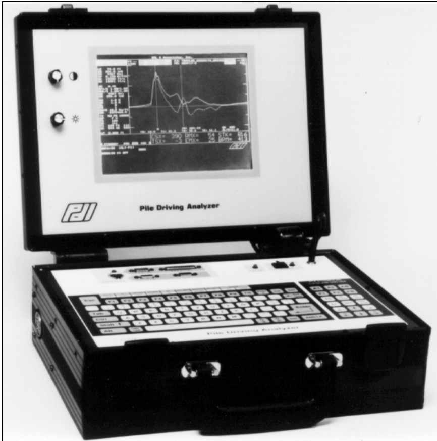
Figure 37, Pile Driving Analyzer, Model PAK (After PDI, 1993)
