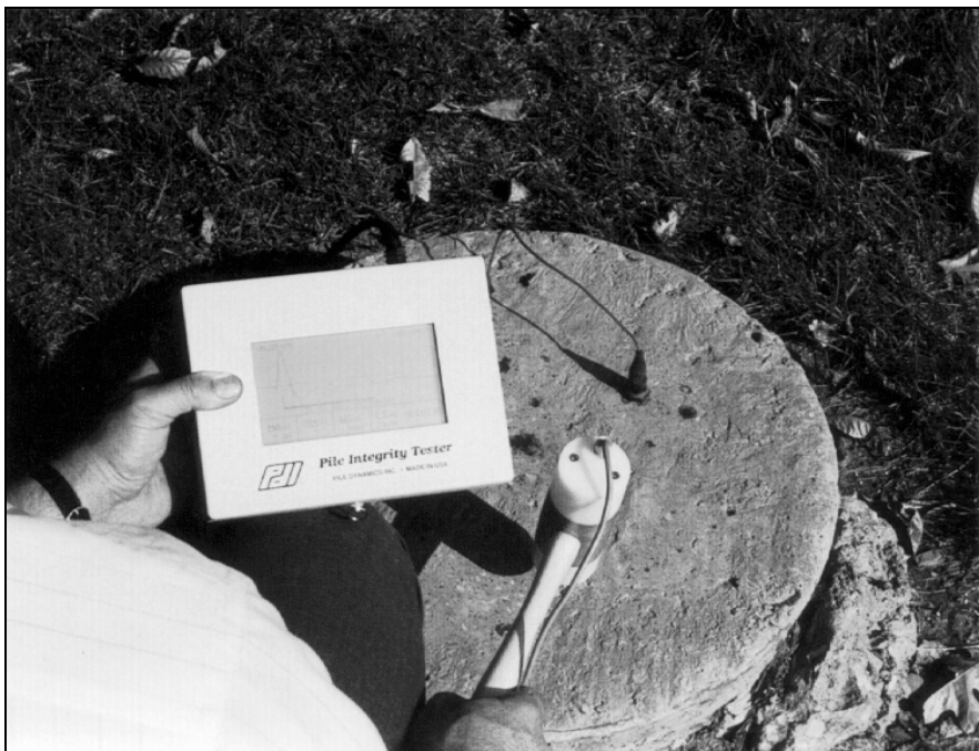
Figure 42, Pile Integrity Tester (After PDI, 1993)
