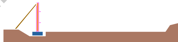
Figure 34, Install & Brace 1st Row of Panels
