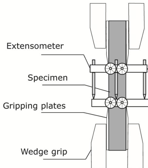
**Figure 65. Illustration. Direct tensile test (DTT) schematic.**
