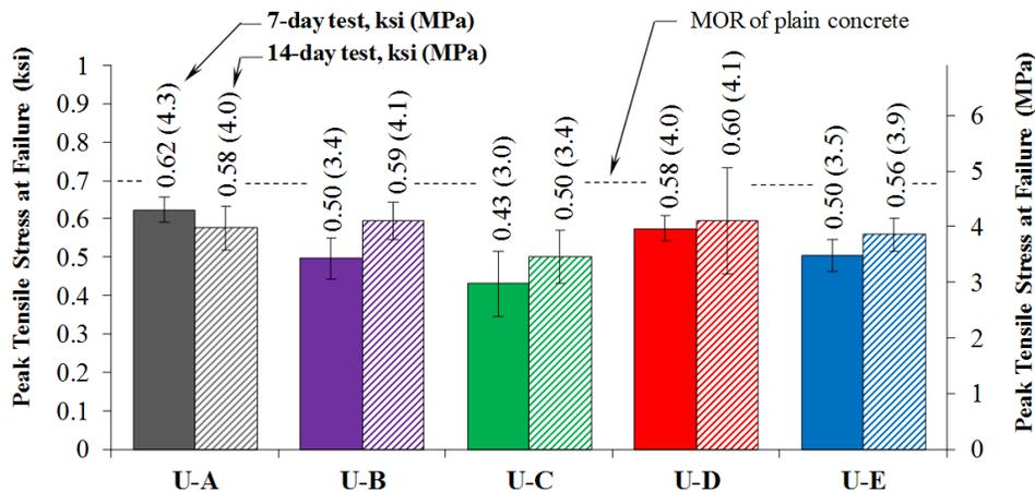
Figure 107. Graph. Results from flexural beam bond tests.
