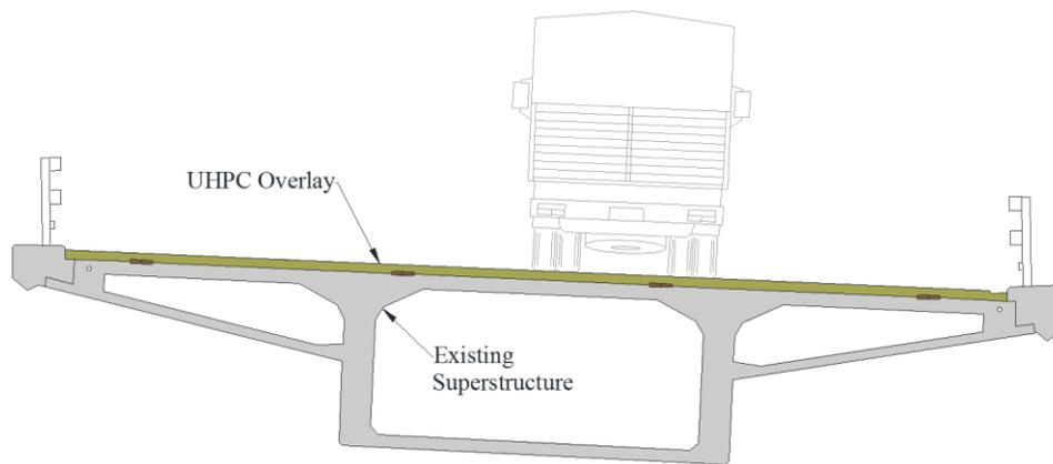
**Figure 6. Illustration. Bridge deck overlay using UHPC.**
