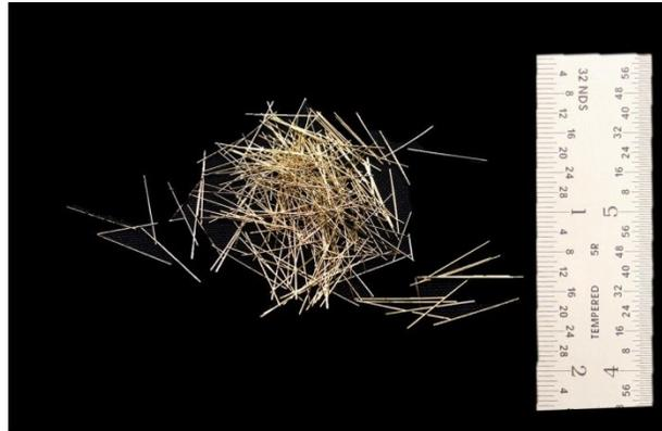
**Figure 14. Photo. of the steel fiber reinforcement used in U-C.**
