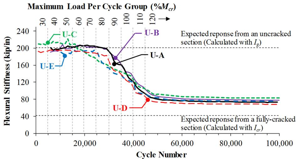
**Figure 161. Graph. Stiffness degradation during pre-cracking cyclic loading.**
