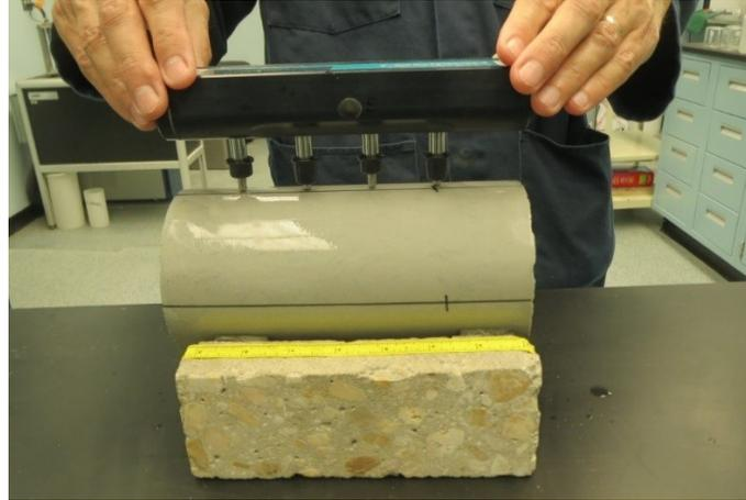
**Figure 129. Photo. Setup for surface resistivity test.**
