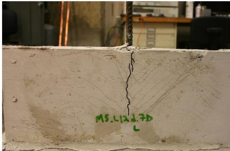
Figure 142. Photo. Bond test failure due to side splitting.
