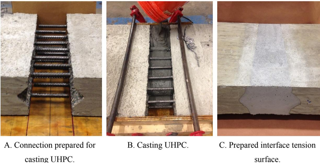
**Figure 154. Photos. Specimen construction and preparation for testing.**
