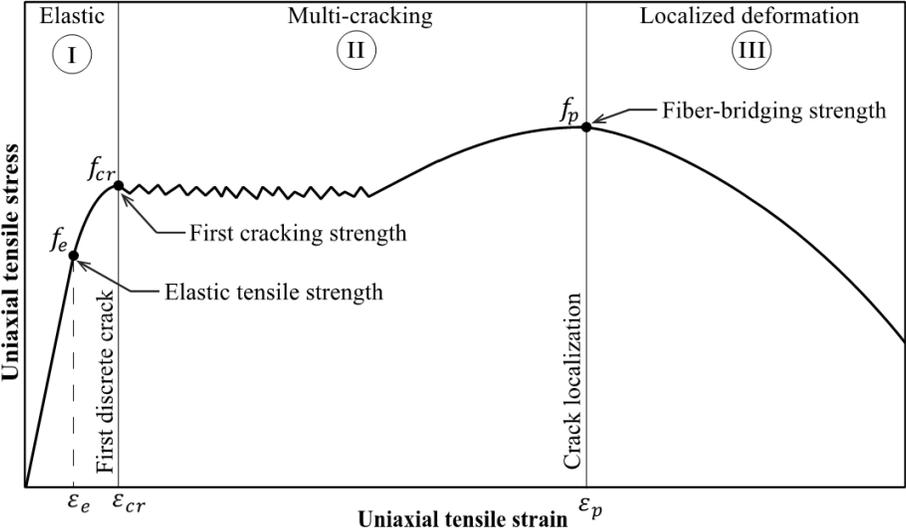
**Figure 67. Illustration. Idealized uniaxial tensile response for UHPC.**
