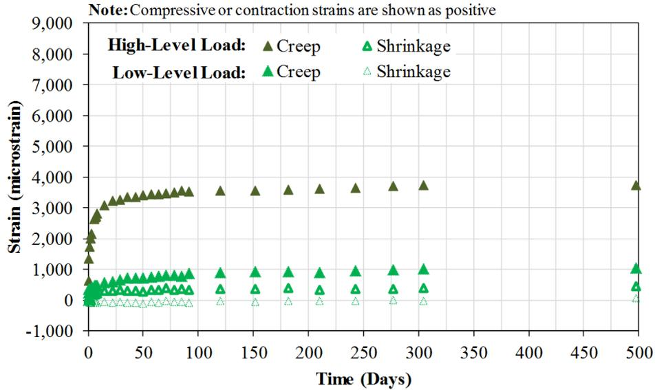
Figure 116. Graph. Creep and shrinkage of U-C.
