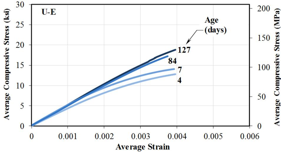
**Figure 42. Graph. Compressive stress-strain response of material U-E.**
