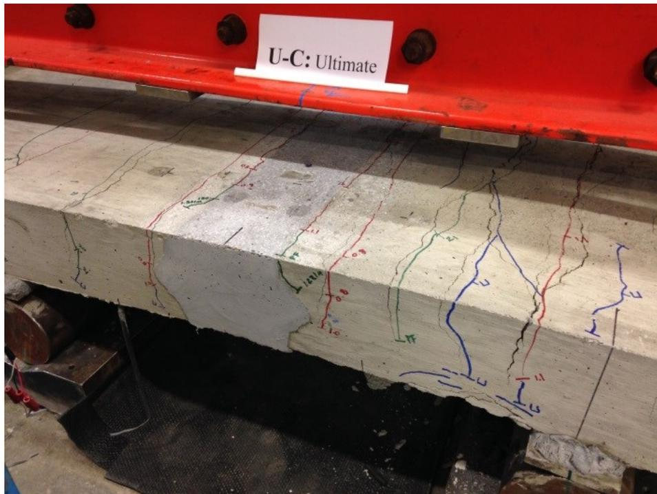
**Figure 182. Photo. Specimen U-C after ultimate loading.**
