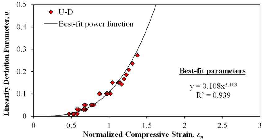
Figure 50. Graph. Deviation from the linear elastic compressive behavior for U-D.
