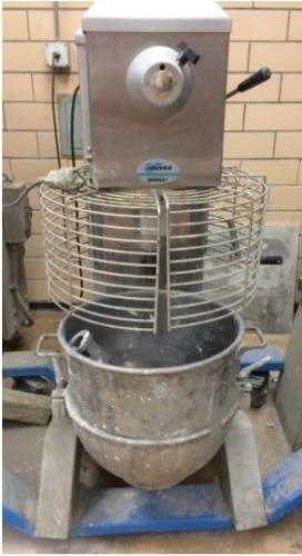
**Figure 18. Photo. Planetary bowl and paddle mixer for UHPC batches up to 0.75 ft<sup>3</sup> (0.02 m<sup>3</sup>).**
