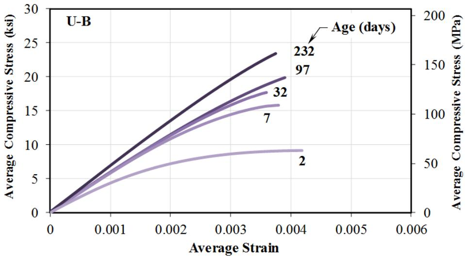
Figure 39. Graph. Compressive stress-strain response of material U-B.
