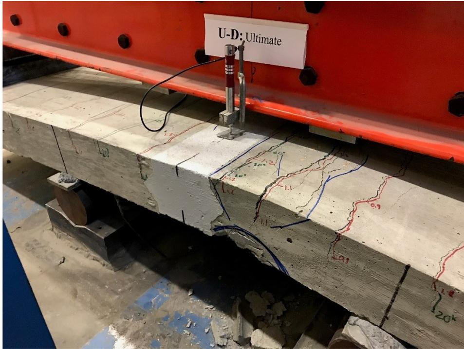
**Figure 183. Photo. Specimen U-D after ultimate loading.**
