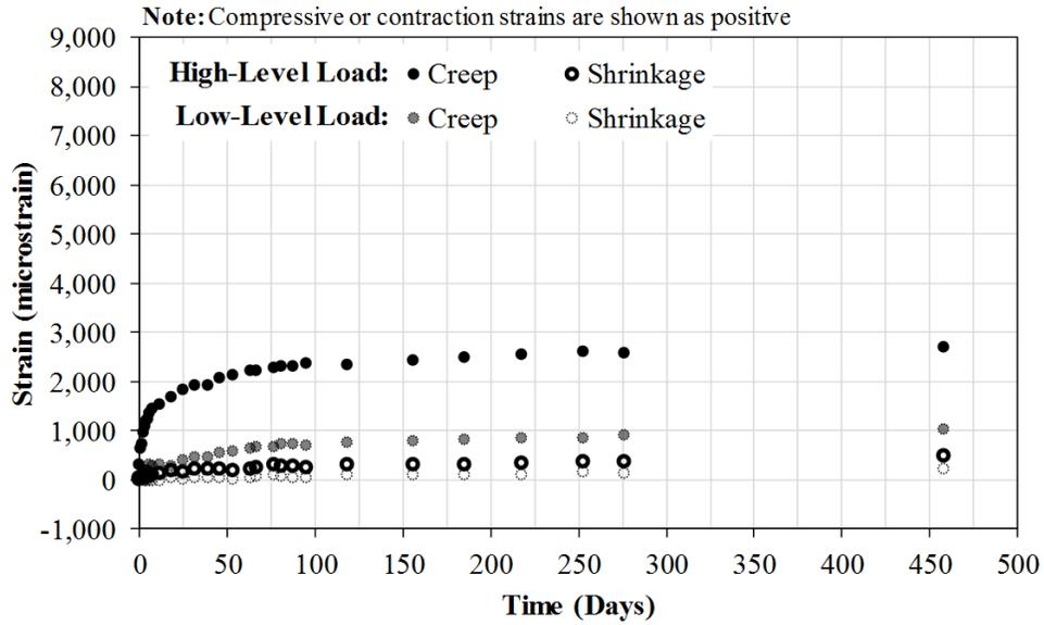
Figure 114. Graph. Creep and shrinkage of U-A.
