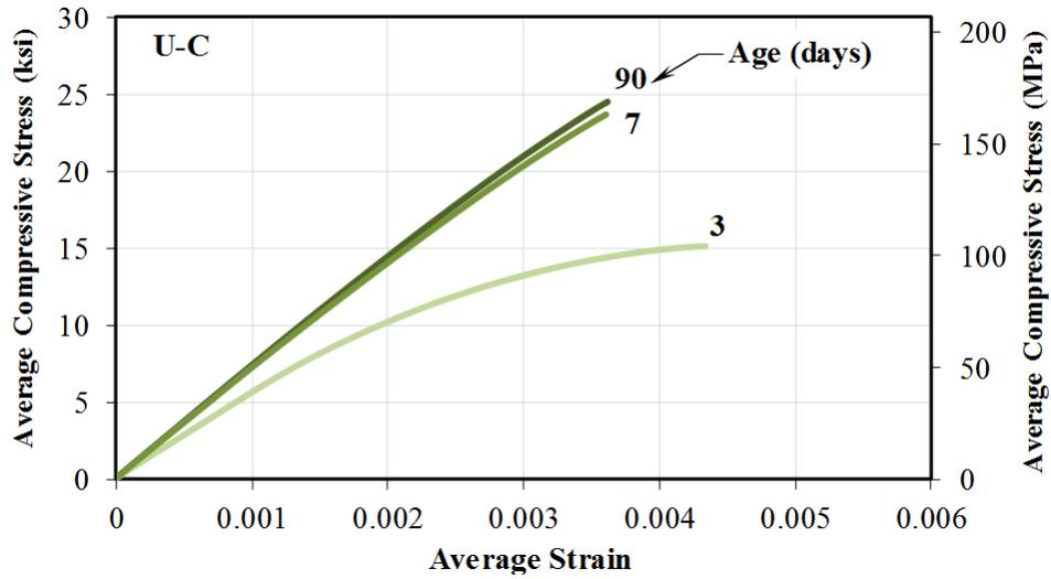
Figure 40. Graph. Compressive stress-strain response of material U-C.
