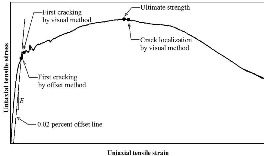
**Figure 73: Illustration. Typical stress-strain relationships of a tensile test specimen exhibiting tension hardening behavior.**
