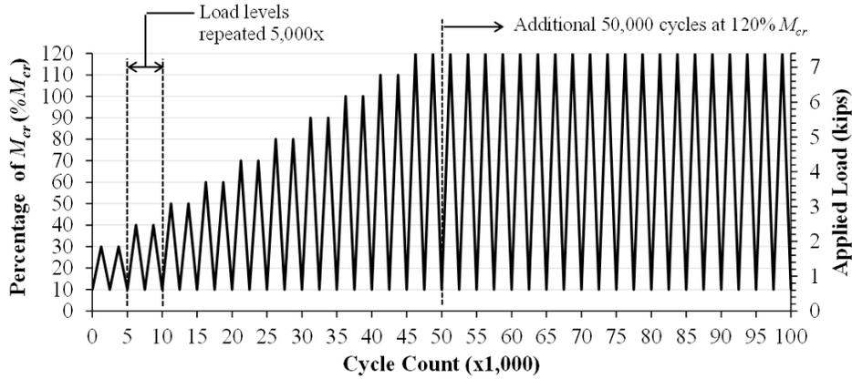
**Figure 156. Graph. Cyclic crack loading protocol (1 kip = 4.448 kN).**
