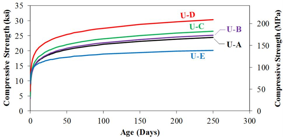
Figure 37. Graph. Compressive strength gain trendlines for UHPCs with 2 percent fiber.
