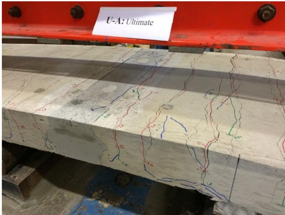
Figure 180. Photo. Specimen U-A after ultimate loading.
