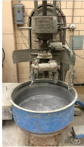
**Figure 19. Photo. Small pan-style mixer for UHPC batches up to 1.0 ft<sup>3</sup> (0.028 m<sup>3</sup>).**
