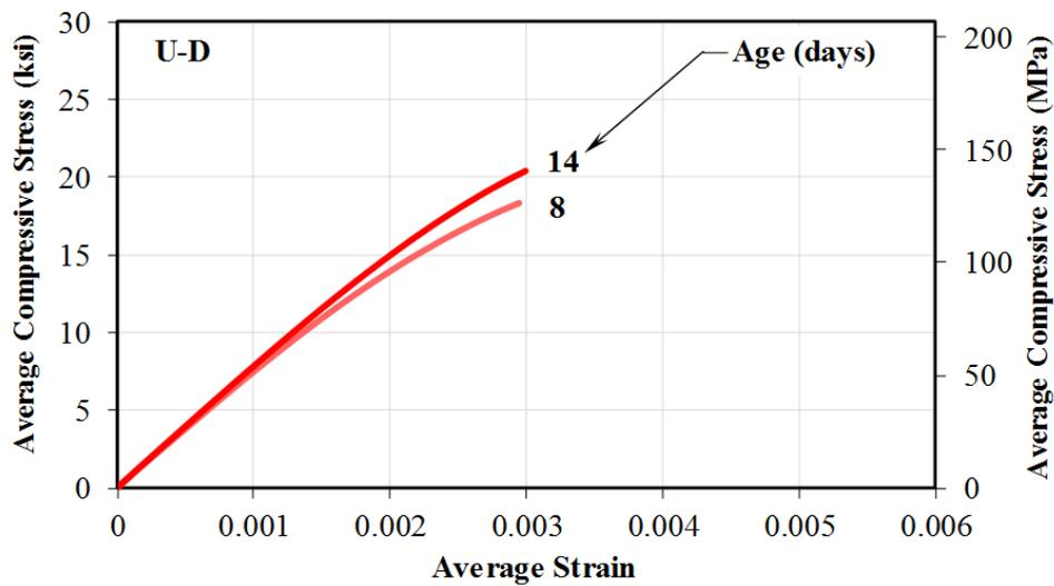
Figure 41. Graph. Compressive stress-strain response of material U-D.
