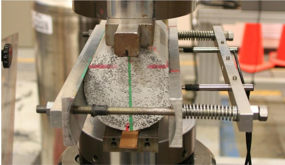
**Figure 95. Photo. Split cylinder tension test (SCTT).**
