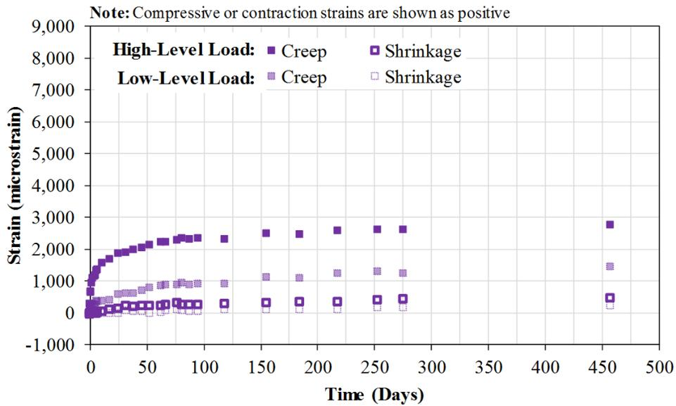
Figure 115. Graph. Creep and shrinkage of U-B.
