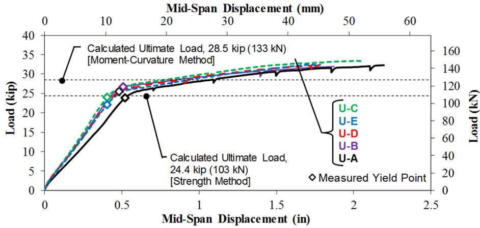
Figure 177. Graph. Force-displacement relationships during ultimate loading.
