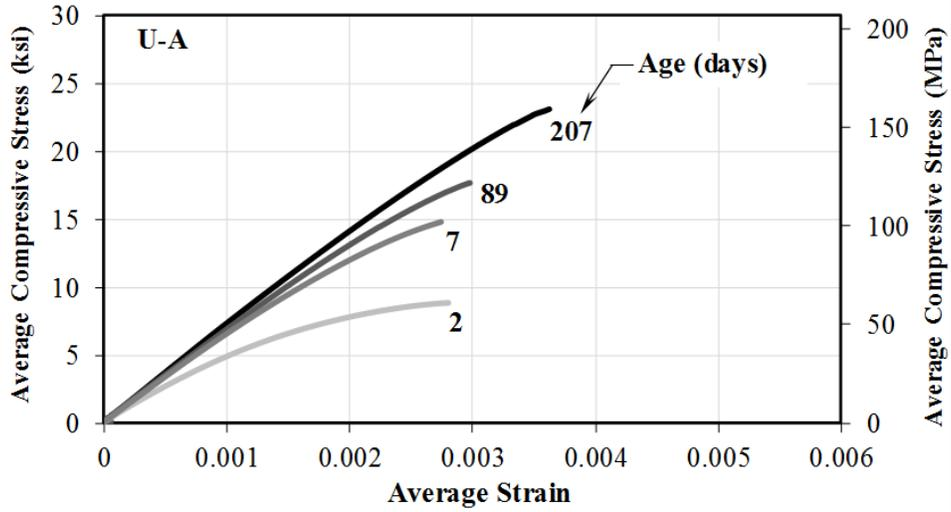
Figure 38. Graph. Compressive stress-strain response of material U-A.
