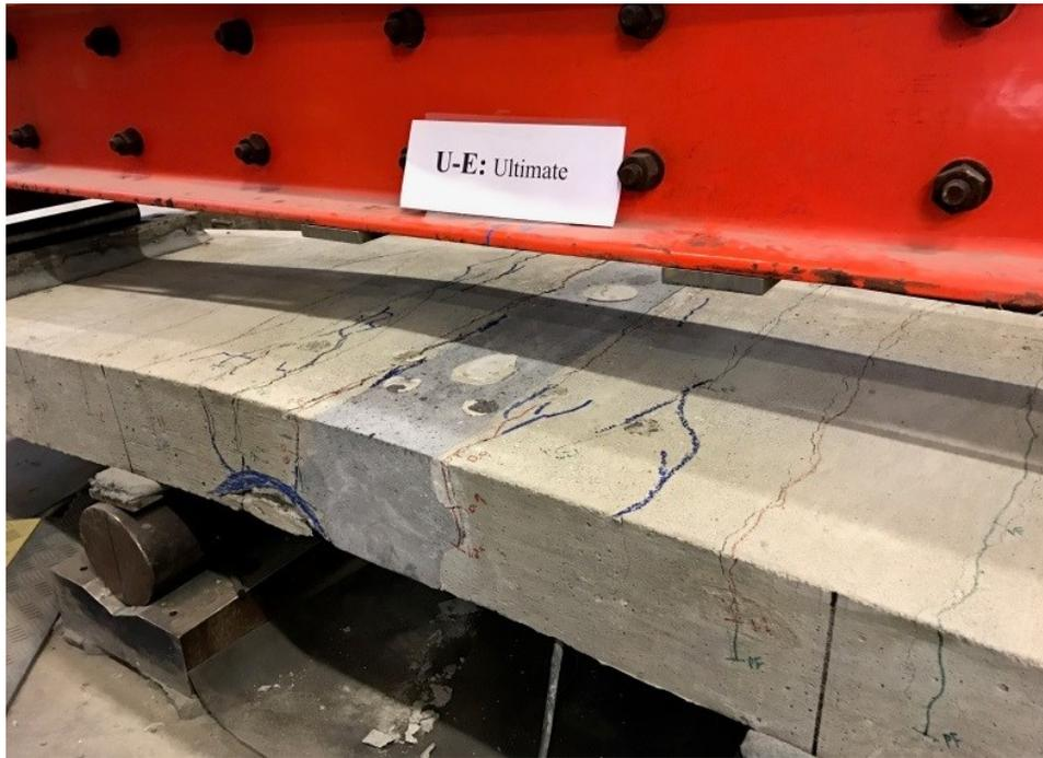
**Figure 184. Photo. Specimen U-E after ultimate loading.**
