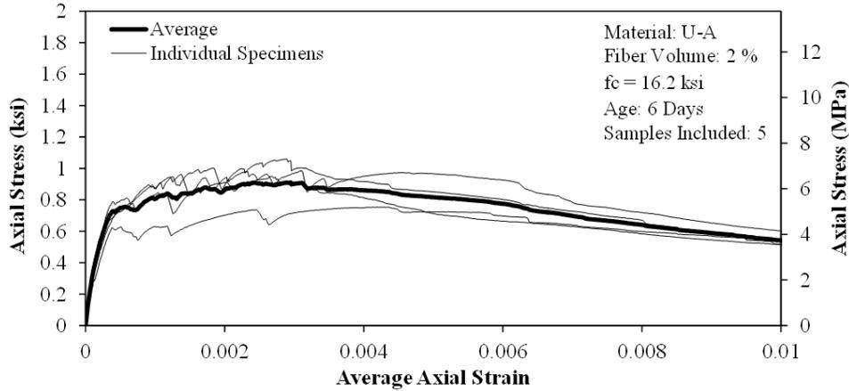
**Figure 74. Graph. Tensile stress-strain response of U-A samples with 2 percent fiber volume.**
