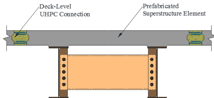
C. UHPC connections between modular superstructure element.
