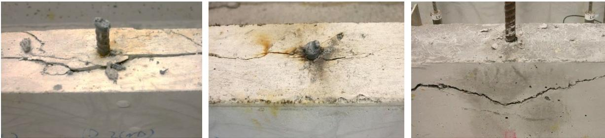
A. Wide splitting cracks: U-D with  $V_f = 1.5$  percent    B. Thin splitting cracks: U-D with  $V_f = 2.5$  percent    C. Cone failure: U-C with  $V_f = 4.5$  percent
