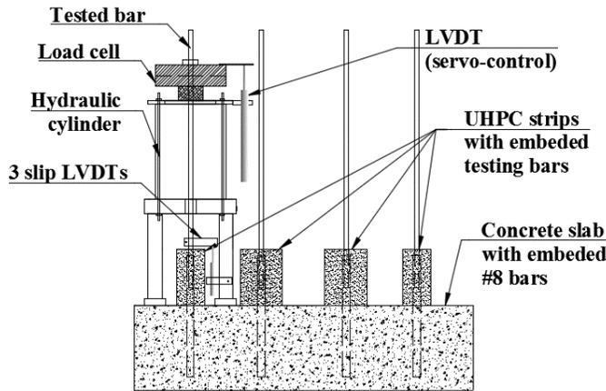
**Figure 136. Illustration. Details of bond pull-out test set-up.**
