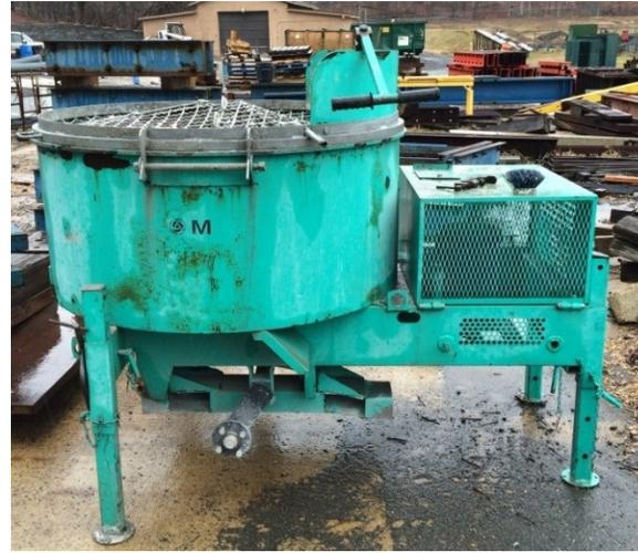
**Figure 20. Photo. Large pan-style mixer with orbital mixing action for UHPC batches up to 4.0 ft<sup>3</sup> (0.11 m<sup>3</sup>).**
