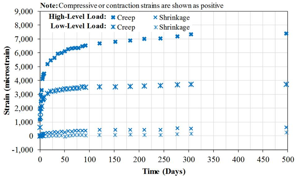
Figure 117. Graph. Creep and shrinkage of U-E.
