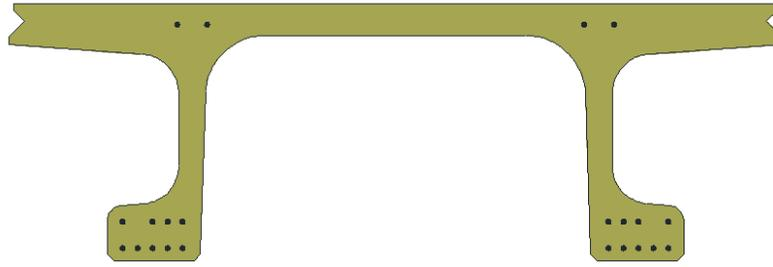
**Figure 11. Illustration. Precast, prestressed UHPC pi-girder element.**
