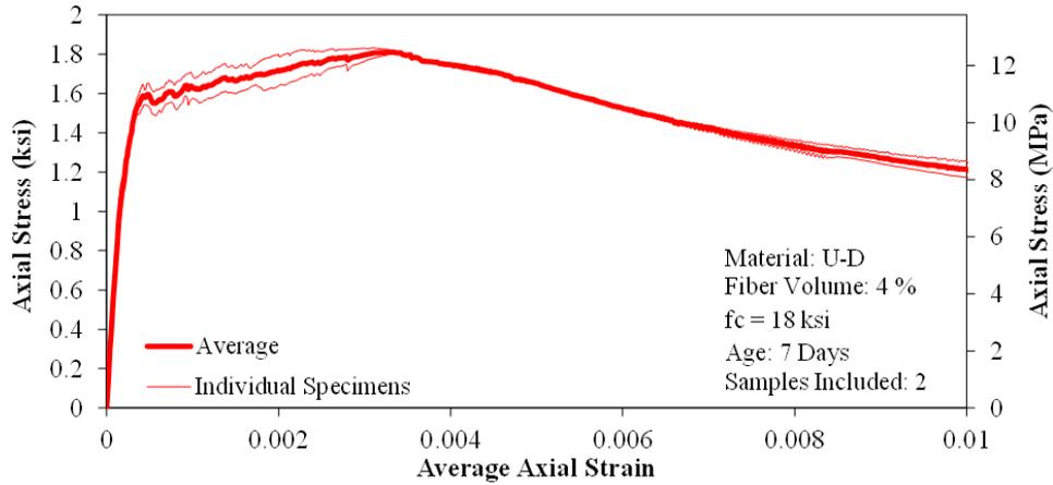
**Figure 85. Graph. Tensile stress-strain response of U-D samples with 4 percent fiber volume after 7 day of curing.**
