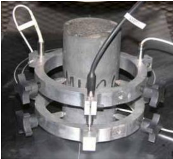
Figure 2-27: Concrete specimen with extensometer for modulus testing (Graybeal 2006)
