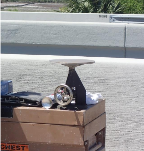
Figure 2-33: Flow table used during UHPC field placement
