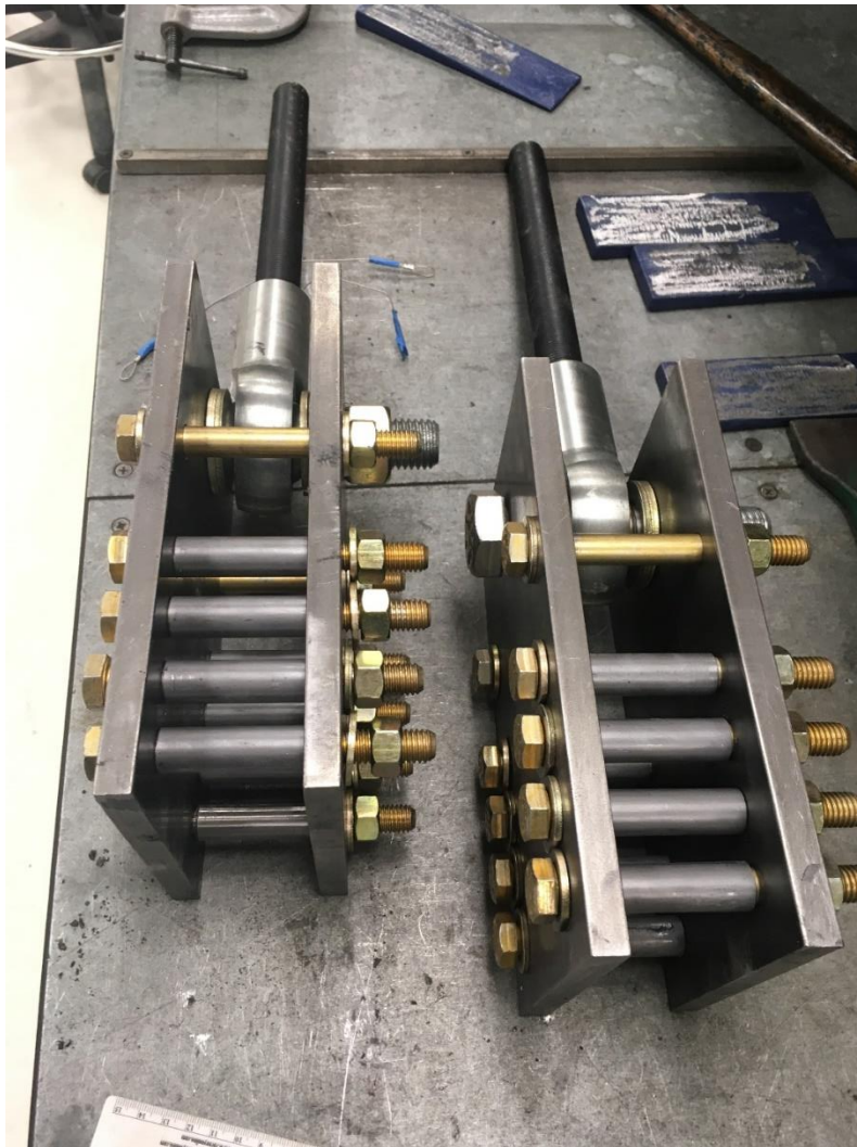
Figure 4-12: SMO direct tension test grips and wedge plates
