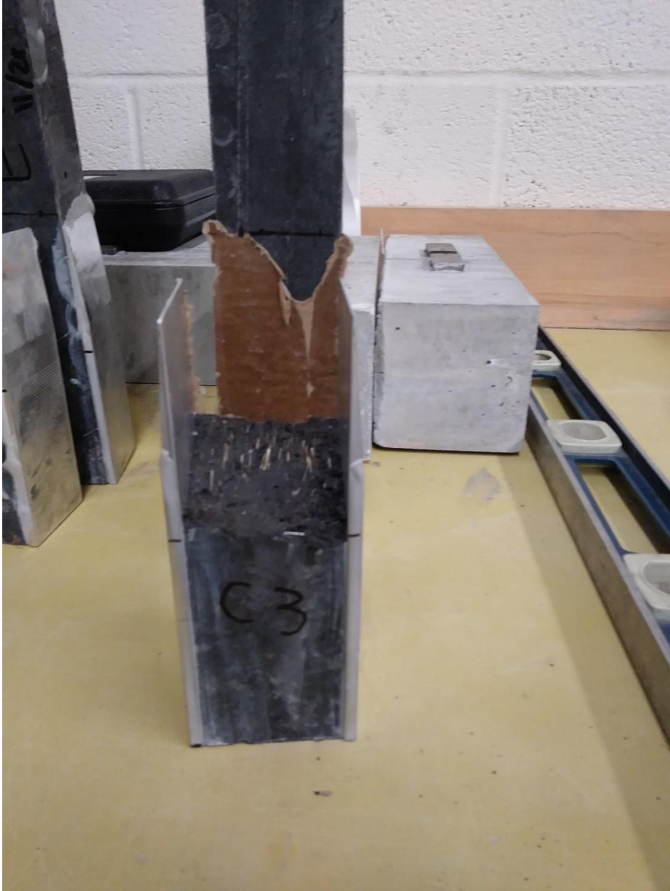
Figure 4-4: Invalid direct tension sample after failure
