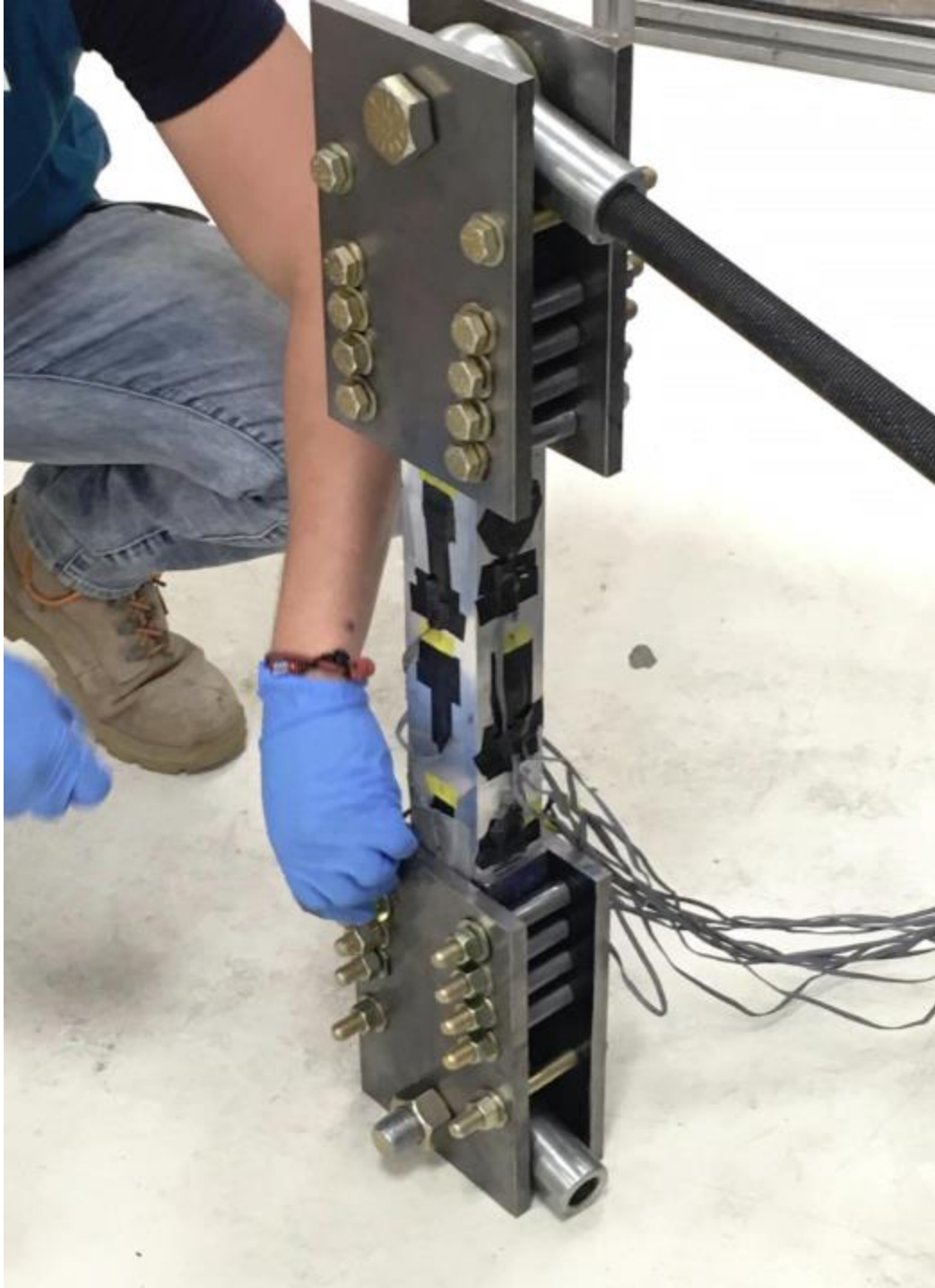
Figure 4-10: Aluminum Specimen in Tensile Grips
