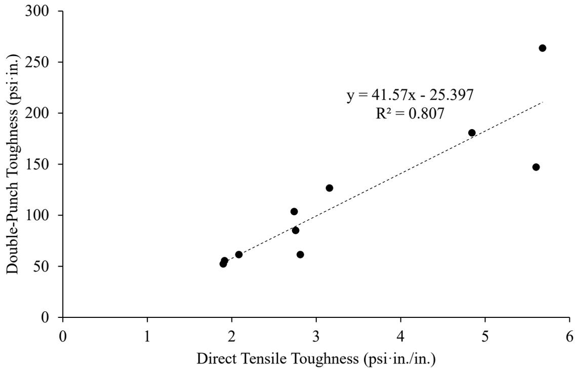
Figure 1-18: Relationship between flexural toughness and direct tensile toughness
