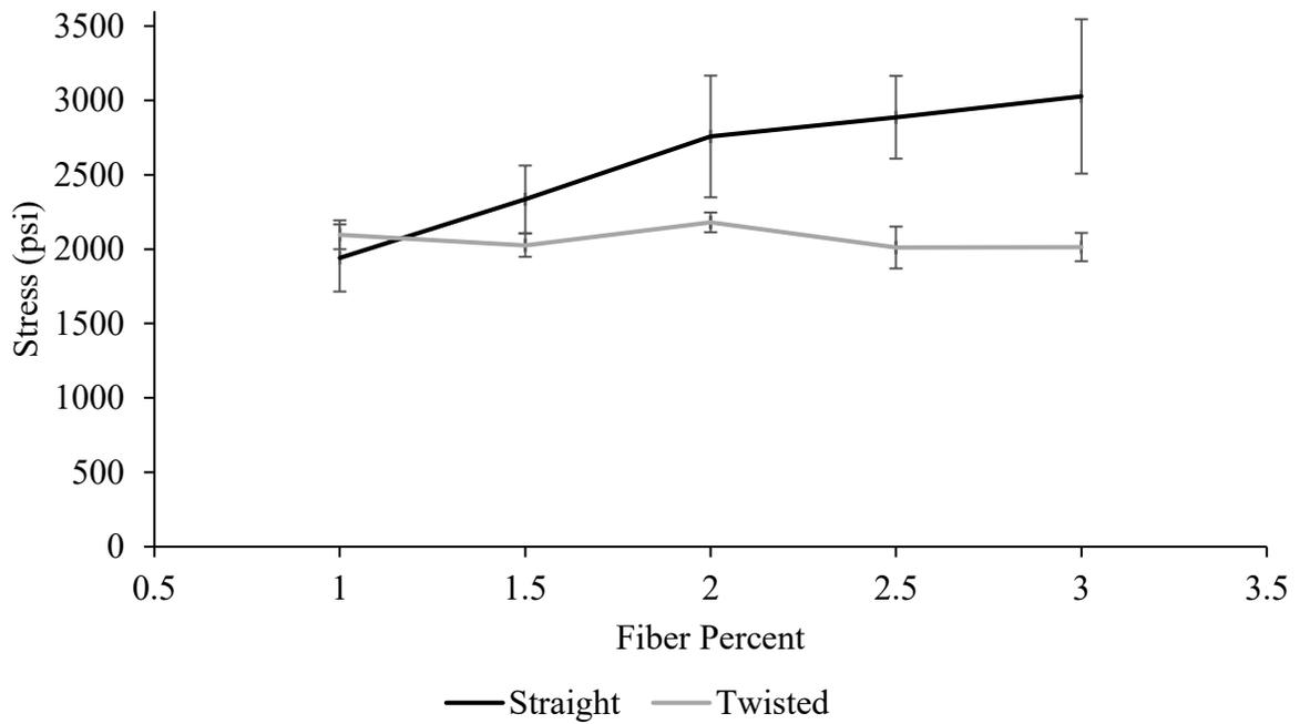
Figure 1-6: Average maximum bending stresses (moduli of rupture) from flexure testing
