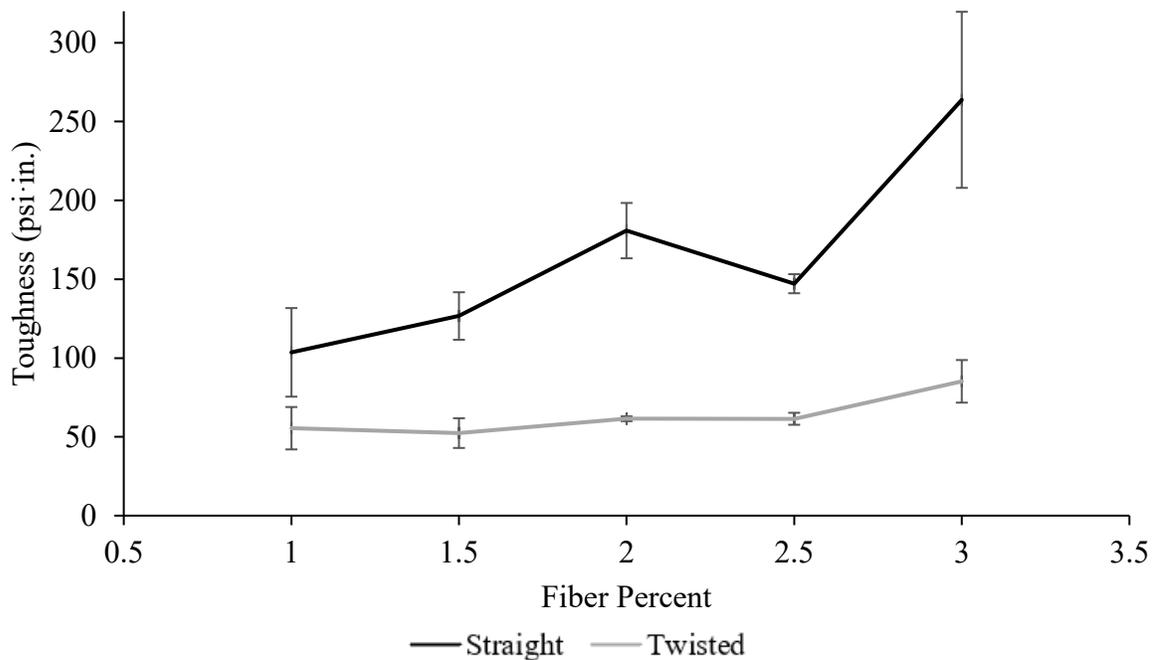
Figure 1-10: Average toughness from double-punch testing
