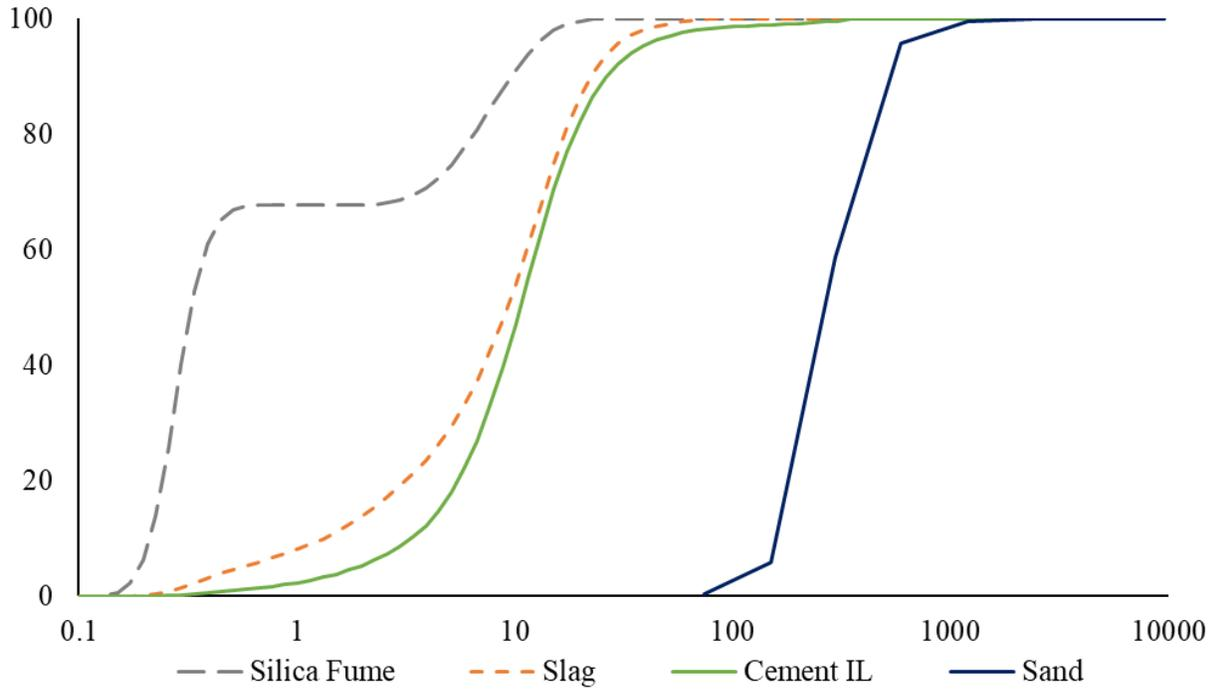
Figure 1-1: Particle size distribution of aggregate and cementitious materials used
