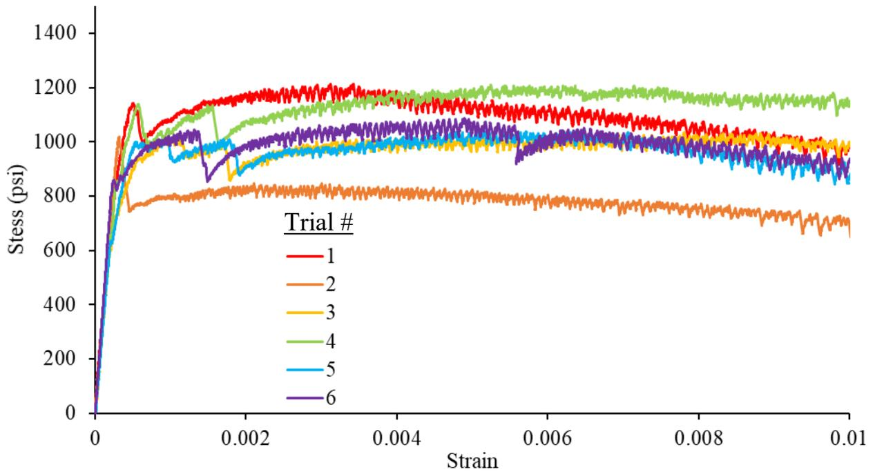
Figure A-23: Direct tension results for 2% straight fiber specimens
