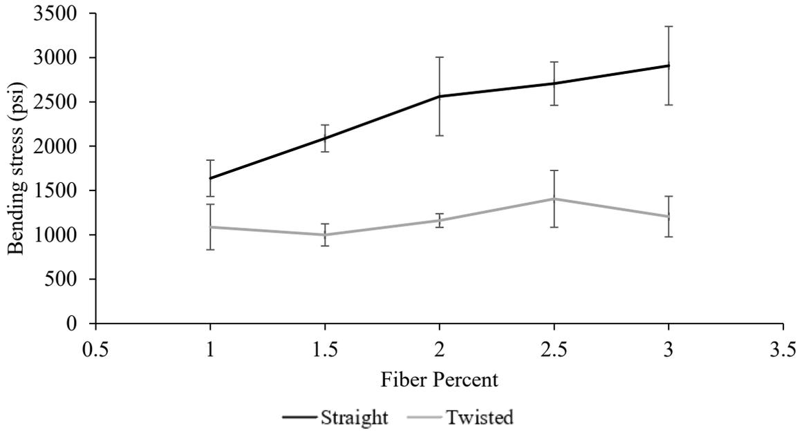
Figure 1-12: Average flexural stress at a deflection of 1/600
