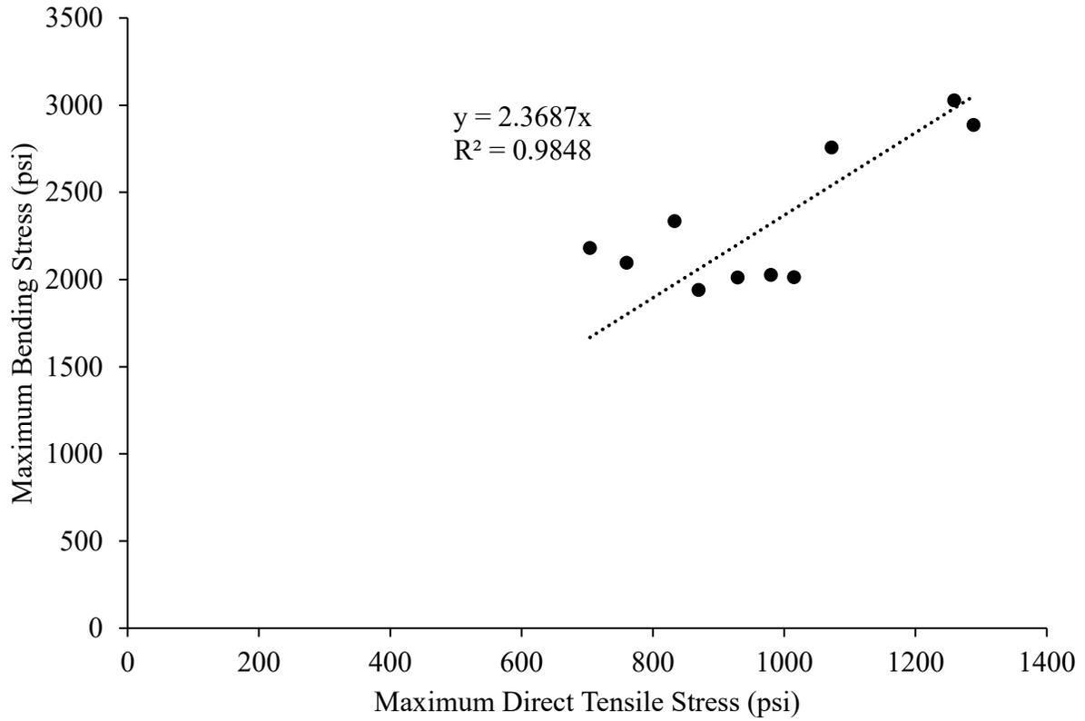
Figure 1-15: Relationship between maximum bending stress in ASTM C1609 and maximum direct tensile stress for specimens tested
