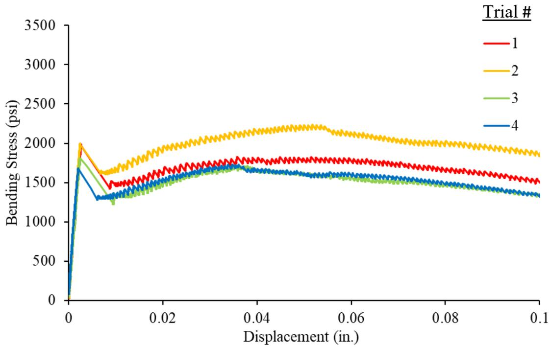
Figure A-11: Flexure results for 1% straight fiber specimens
