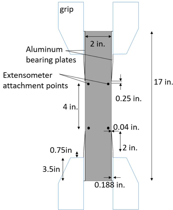
Figure 1-2: Direct tension testing set-up
