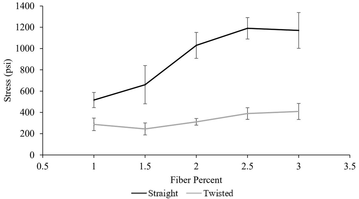
Figure 1-11: Average direct tensile stress at 0.005 in./in. strain
