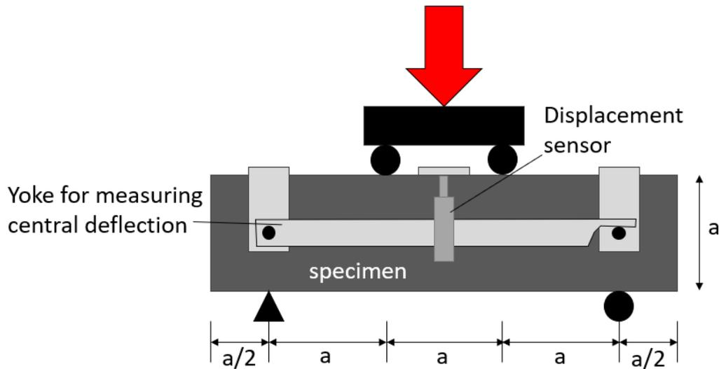
Figure 1-3: Flexure testing set-up
