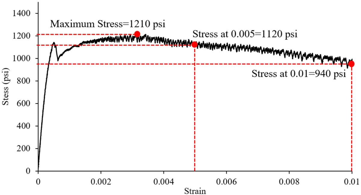
Figure 1-22: Example of qualification values taken from a direct tension test
