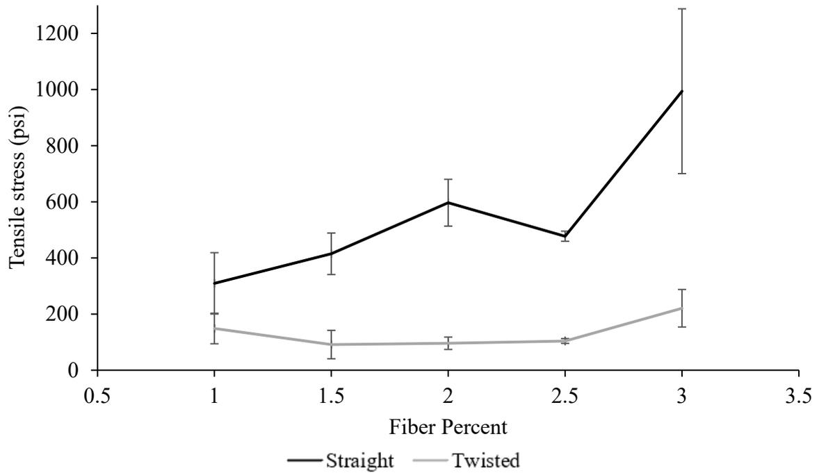
Figure 1-14: Average double-punch tensile stress at a vertical displacement of 0.14 inches
