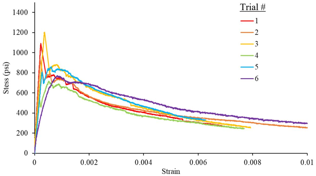
Figure A-29: Direct tension results for 2.5% twisted fiber specimens
