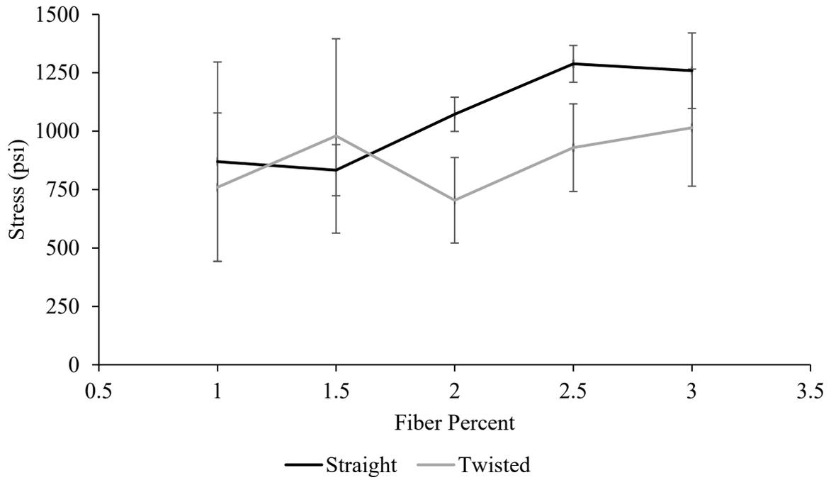
Figure 1-5: Average maximum stresses from direct tension testing
