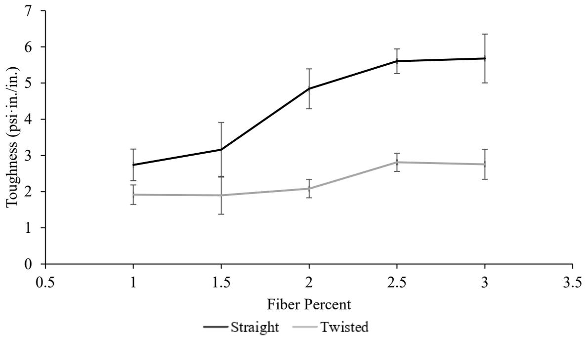
Figure 1-8: Average toughness from direct tensile testing
