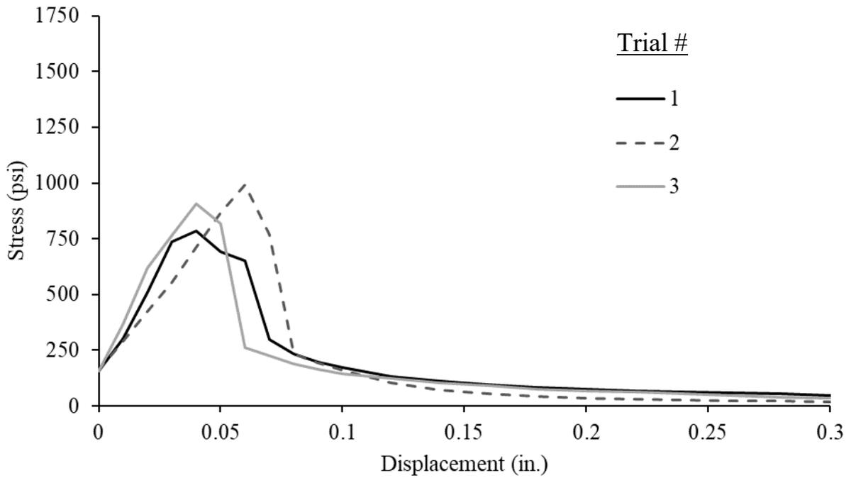
Figure A-8: Double-punch results for 2% twisted fiber specimens
