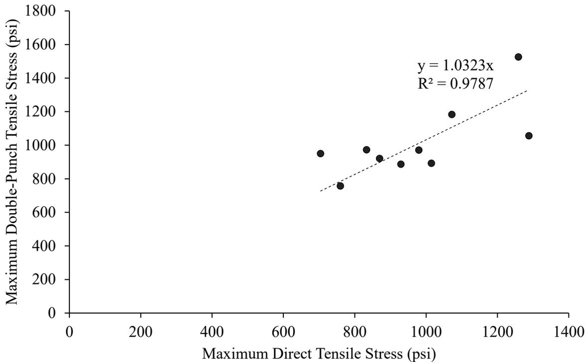
Figure 1-16: Relationship between maximum double-punch tensile stress and maximum direct tensile stress for specimens tested
