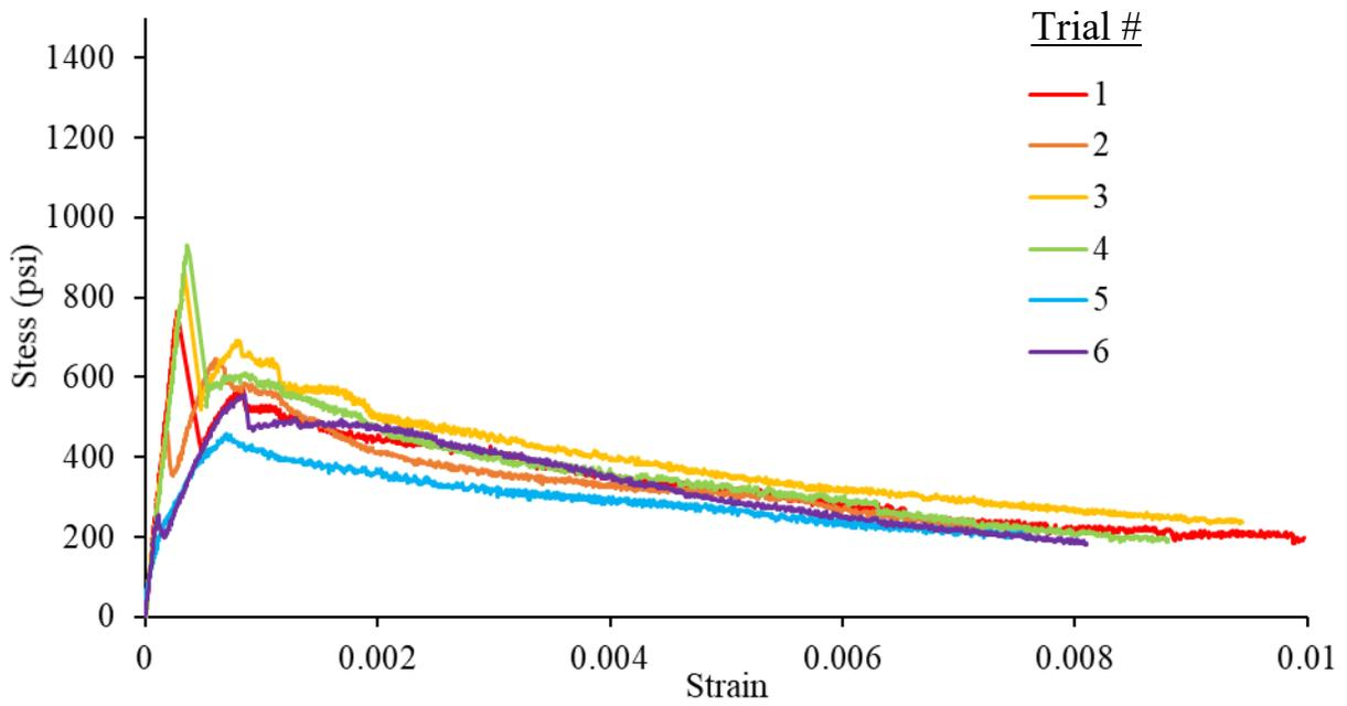
Figure A-28: Direct tension results for 2% twisted fiber specimens
