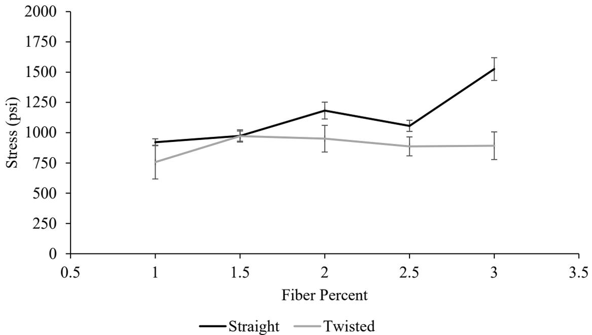
Figure 1-7: Average maximum tensile stress from double-punch testing
