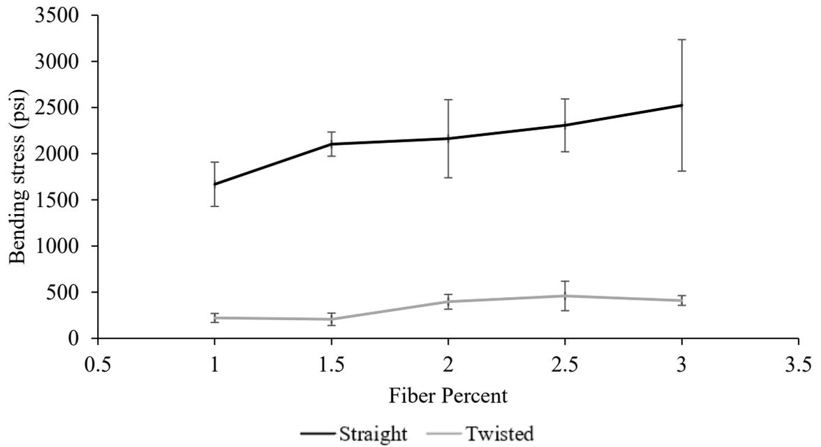
Figure 1-13: Average flexural stress at a deflection of 1/150
