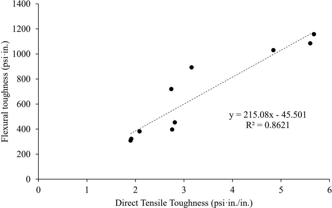
Figure 1-17: Relationship between flexural toughness and direct tensile toughness
