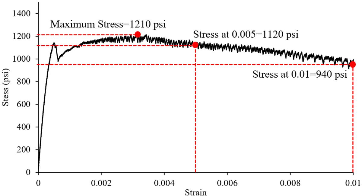
Figure 1-22 shows a schematic of the results from a direct tension test and which points would be
