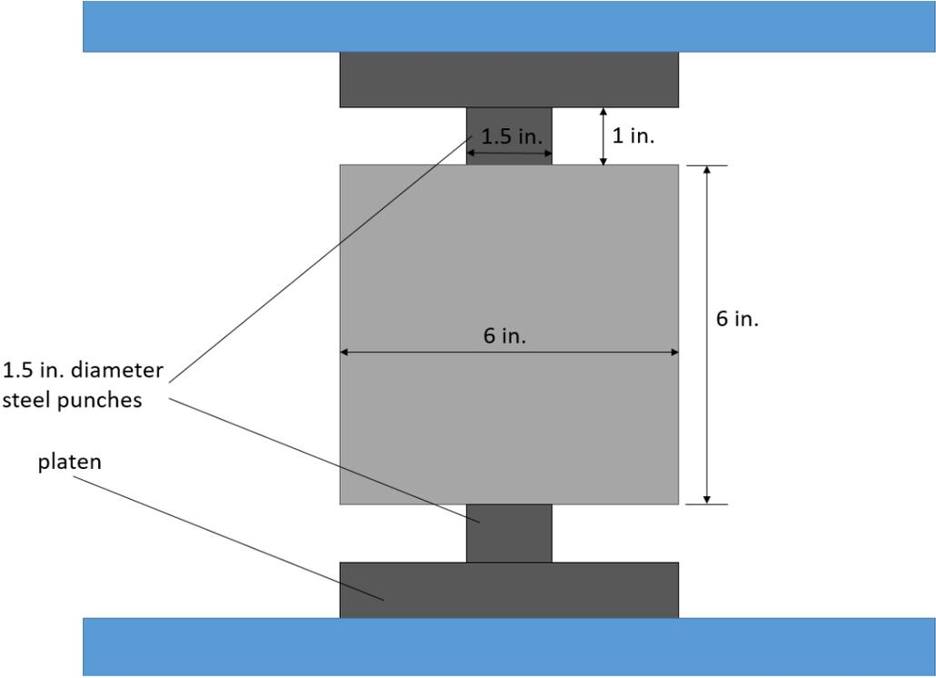
Figure 1-4: Simplified double-punch test set-up
