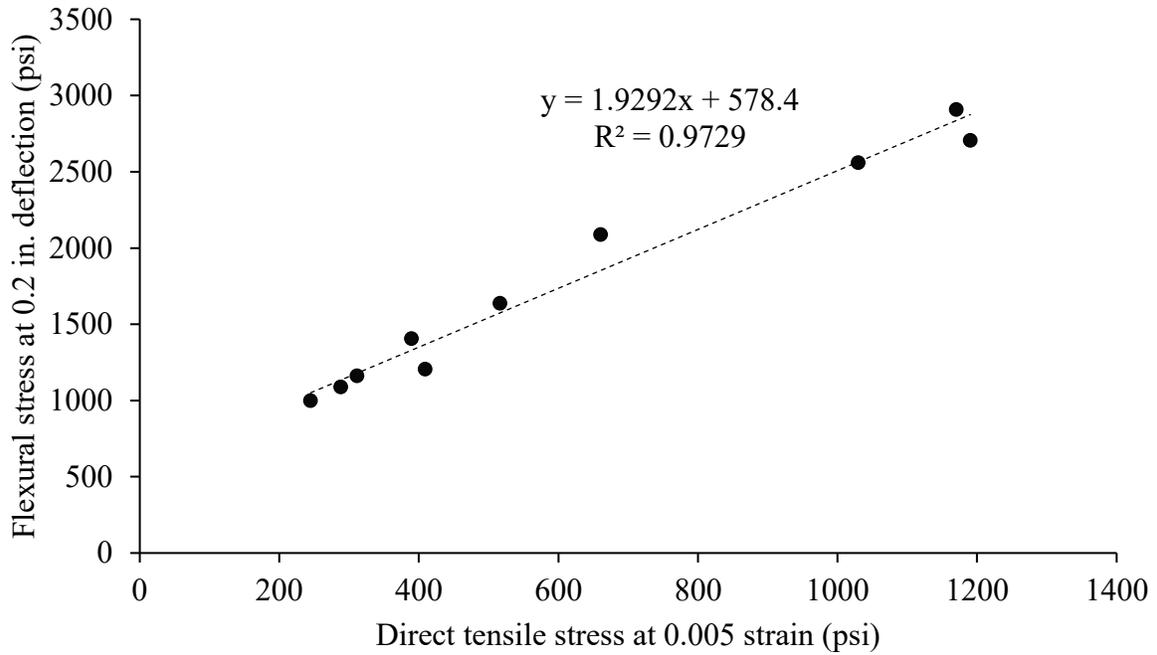
Figure 1-19: Flexural stress at 1/600 (0.2 in.) vs. direct tensile stress at 0.005 strain
