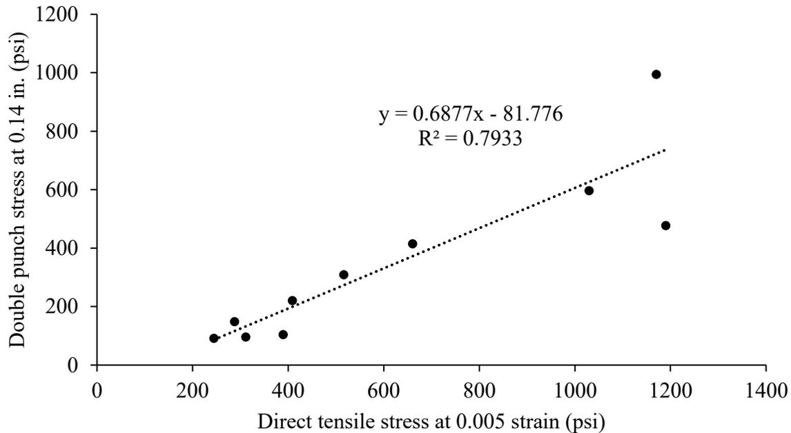
Figure 1-21: Double-punch stress at 0.14 in. vs. direct tensile stress at 0.005 strain
