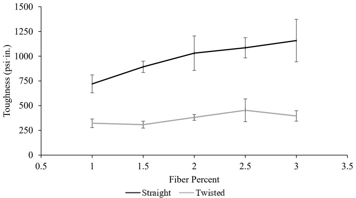
Figure 1-9: Average toughness from ASTM C1609 flexural testing
