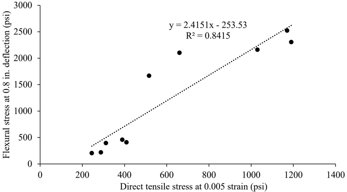
Figure 1-20: Flexural stress at 1/150 (0.8 in.) vs. direct tensile stress at 0.005 strain
