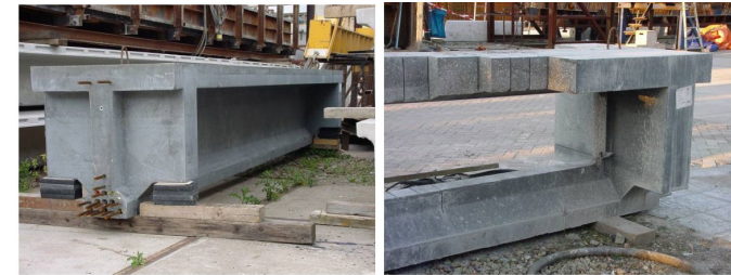
Mock-up of one half of a \pi -shape beam before and after sawing (Simon et al. 2013)
