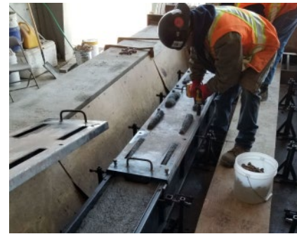
Casting of H-piles in H-direction (photo courtesy: Cor-Tuf)
