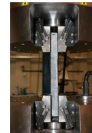
Direct tension 2" x 2" X 17" (11") Stress-strain
