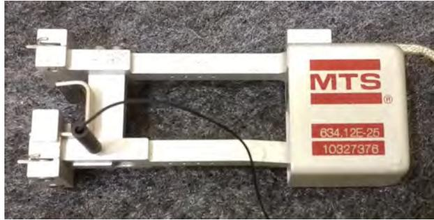
Figure 4.21: MTS extensometer
