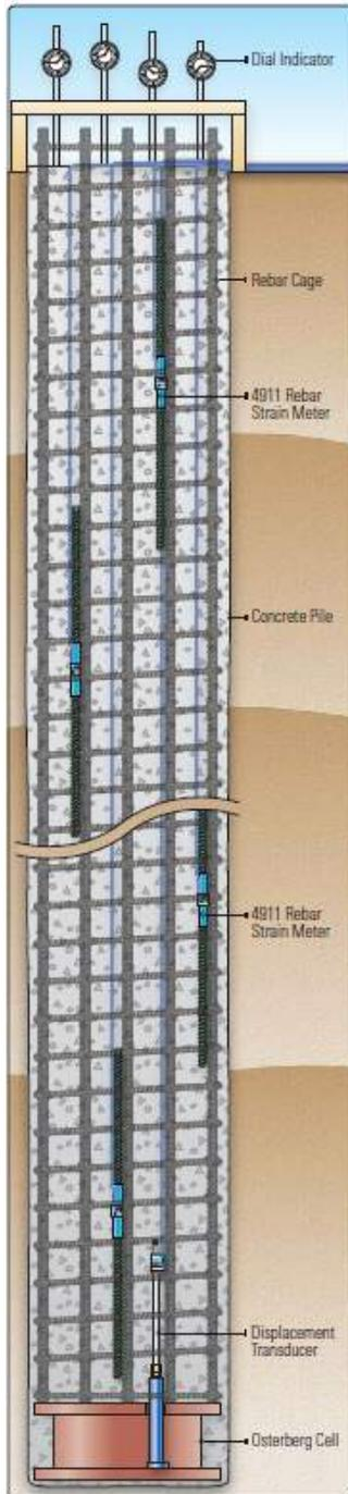
● Installation of the Model 4911 in an Osterberg Cell pile test. (For more information regarding Osterberg Cell pile testing, please contact Inertec Inc. — [www.inertec.com](http://www.inertec.com))
