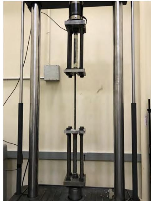
Figure 4.15: Tensile fixture installed in load frame
