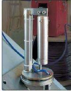
• Model G350 installation using a custom mounting bracket designed for concrete face rock fill dam applications (shown with protective cover removed)
