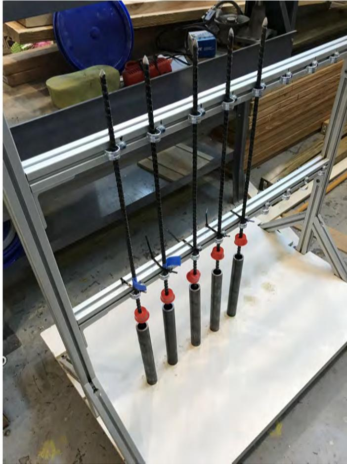
Figure 4.7: Tensile test preparation alignment frame
