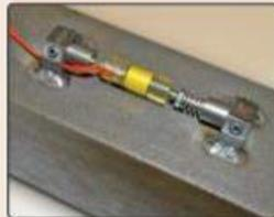
• Model 4150 shown with optional arc-weldable mounting blocks.
