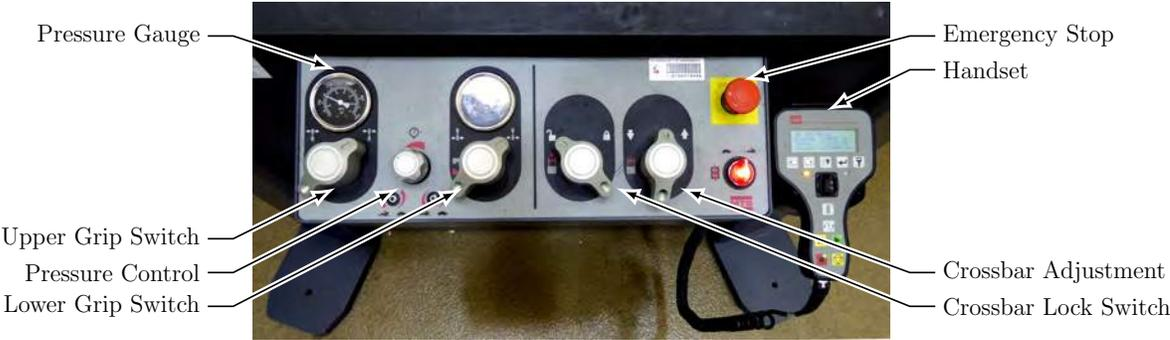
Figure 4.20: MTS control panel
