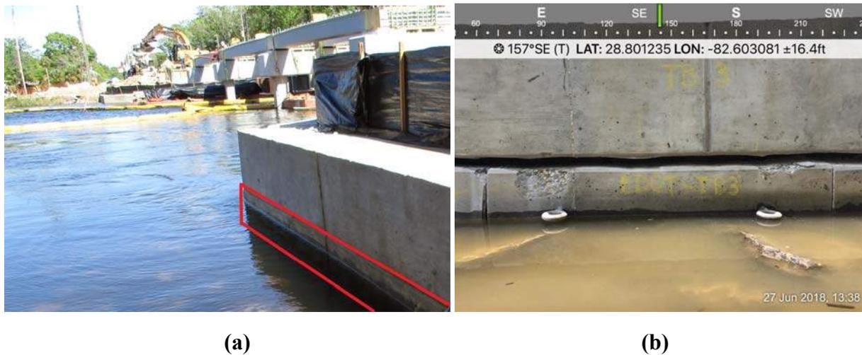
**Fig. 5.** Typical position of test blocks: (a) High tide at HRB (test block outlined); (b) Benchmark test blocks cut and ready for extraction.
