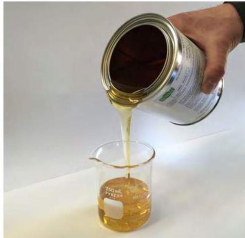
Figure 2.2: Thermoset polymeric resin used in FRP rebars
