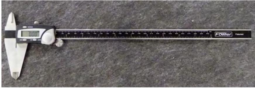
Figure 4.5: Electronic caliper
