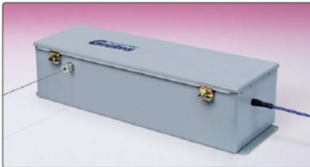
• Model 4427 Long-Range Displacement Meter
