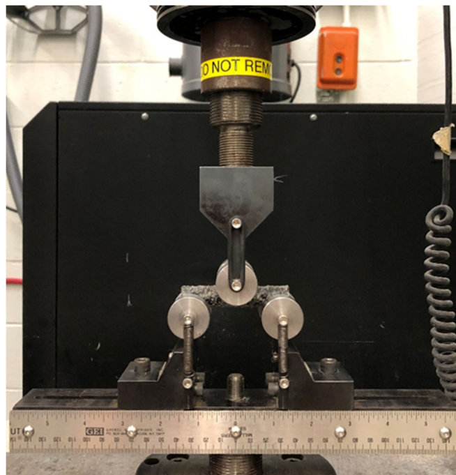
Figure 4.7 – Horizontal shear strength test set-up.
