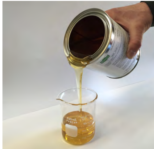
Figure 2.2: Thermoset polymeric resin used in FRP rebars
