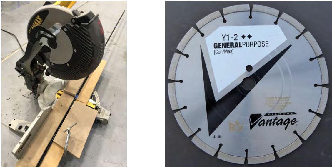
Figure 4.3: Saw and diamond blade for BFRP rebar cutting
