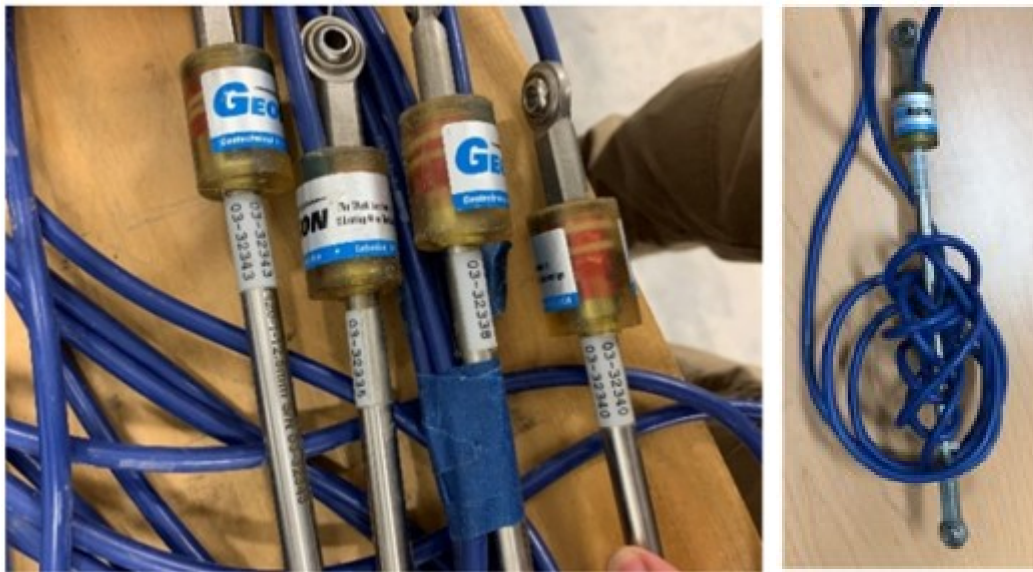
Figure 2.9: External displacement transducers
