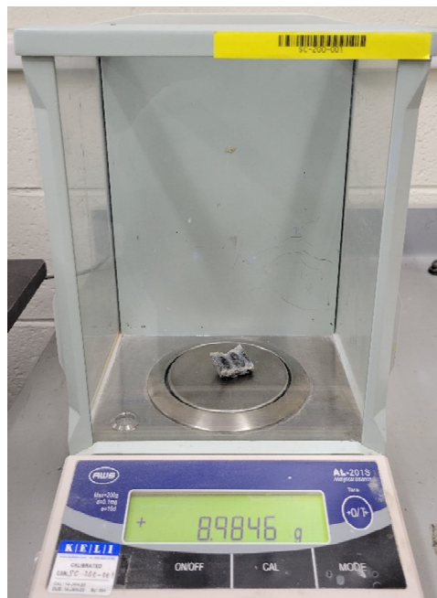
Figure 4.4 – Test set up for measurement of moisture absorption,
