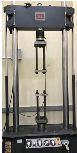
Figure 4.15: Tensile fixture installed in load frame
