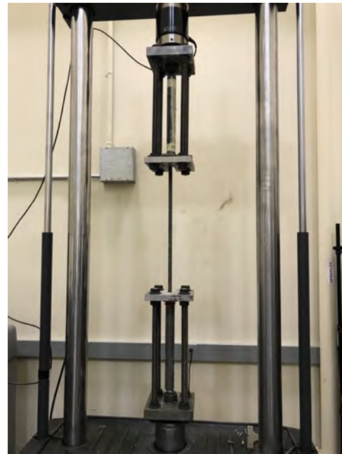
Figure 4.15: Tensile fixture installed in load frame
