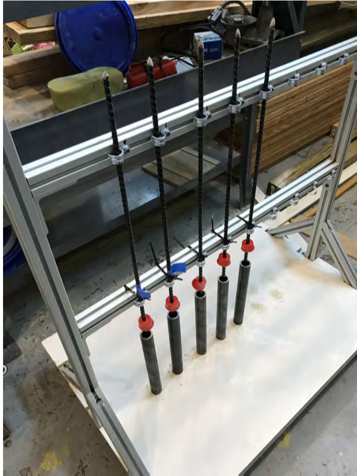
Figure 4.7: Tensile test preparation alignment frame
