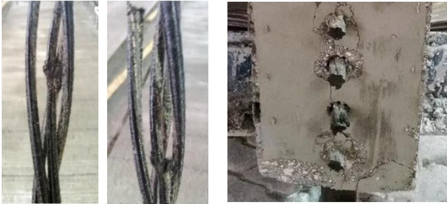
(a) & (b) CFRP strand failed during tensioning; (c) cracking following strands release.
