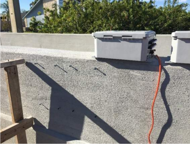
Photo 10 & 11: Installing and setting up data loggers and cable connections
