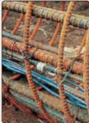
• Close-up of Model 4911 shown as installed in concrete pile reinforcing cage.
