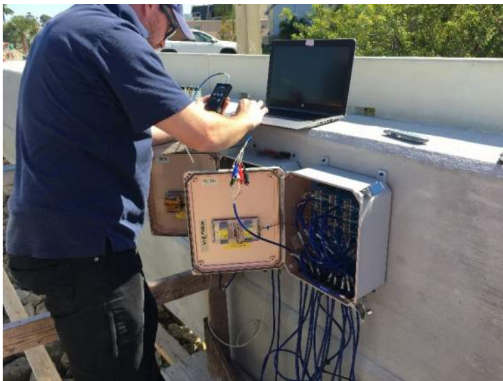
Photo 12: Thomas Fowler (UNF) setting sampling rate and taking baseline readings.
