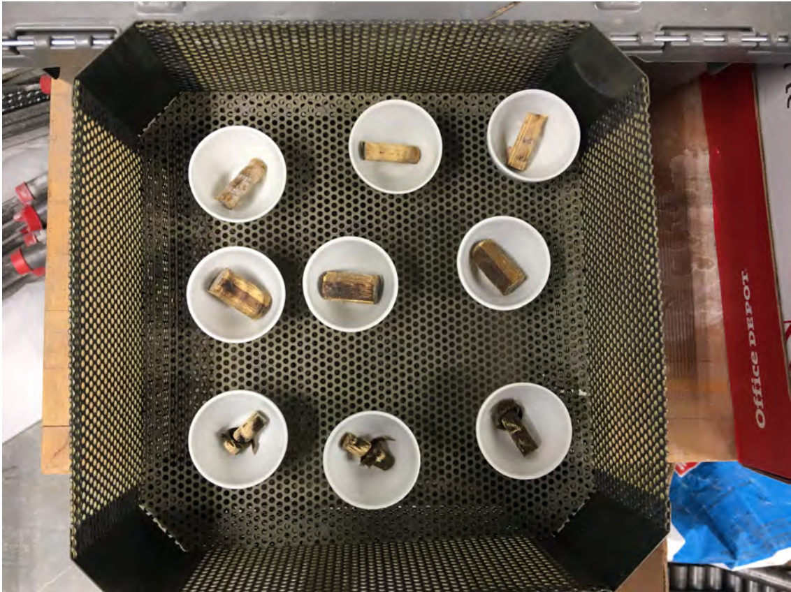
Figure 3.2: Fiber content specimen of GP HP # 3, 5 after test
