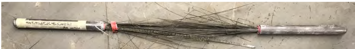
Figure 3.21: GP HP #5, final failure pattern after tensile test
