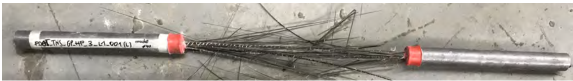
Figure 3.20: GP HP #3, final failure pattern after tensile test
