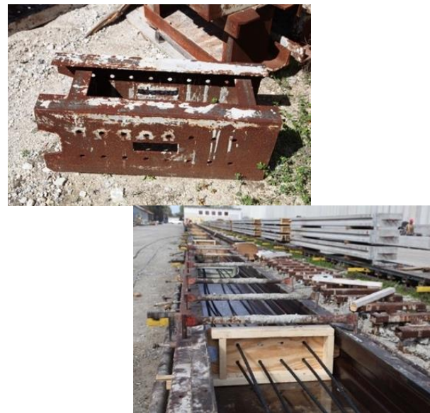
Figure 7-8: Standard steel headers (top) and plywood headers (bottom)
