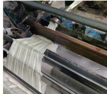
(b) Wetting fibres in the resin bath
