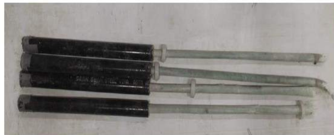
Figure 2 – Typical failure of bent portions the tested MST GFRP bent bars of #6
