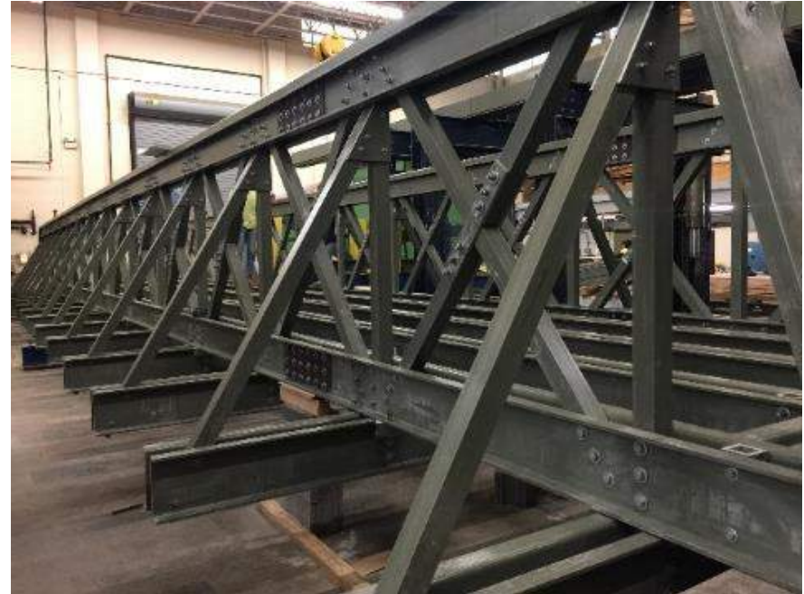
70' long single-span FRP pedestrian bridge being tested at CFC-WVU lab
