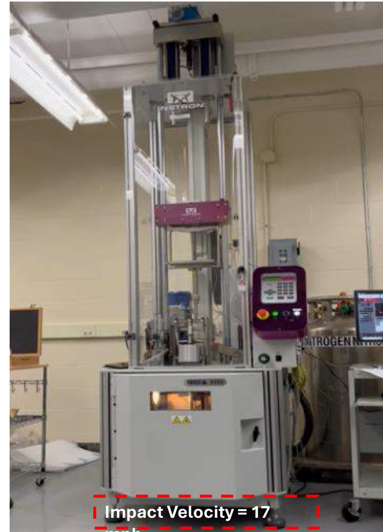
Dynamic impact test (ASTM D7136)
