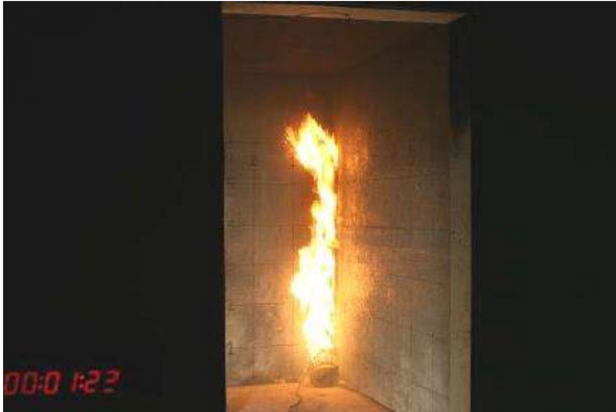
1 min 23 sec into test of four-inch thick composite deck panel as per Test Standard ISO 9705-1993
