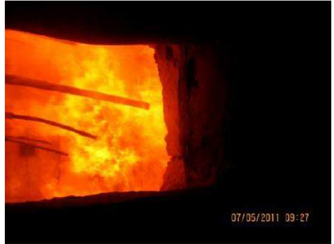
7 min after start of test of a multifunctional non-load-bearing wall panel with intumescent coating as per ASTM E119
