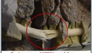
Tension rupture of GFRP bar at failure
