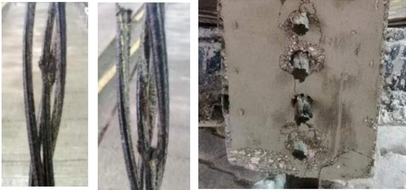
(a) & (b) CFRP strand failure during tensioning;
