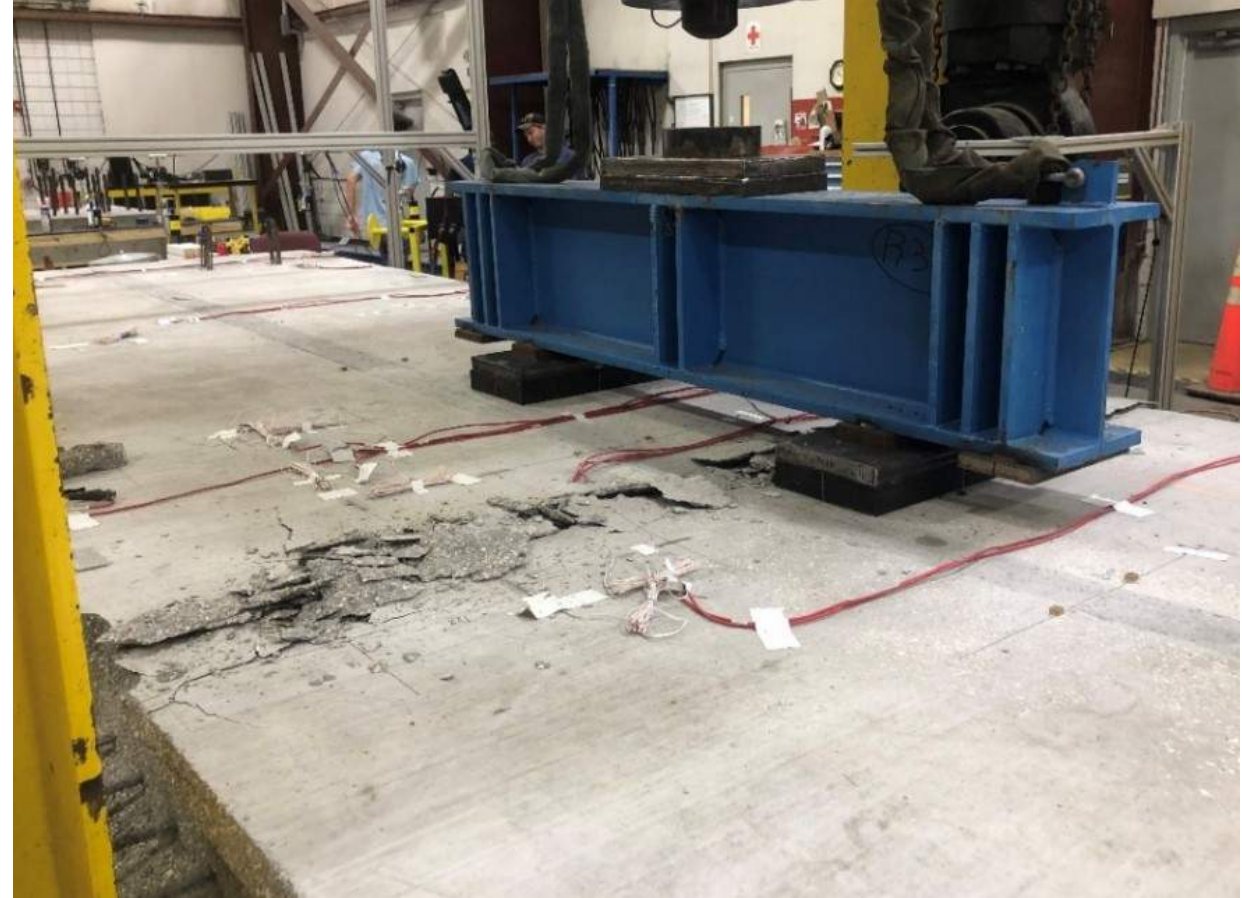
Strength Testing to Evaluate Overall Joint Integrity
