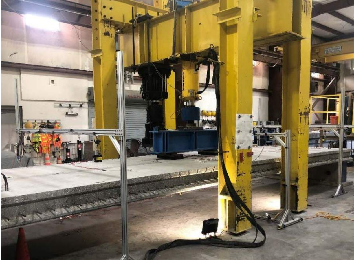
Strength Testing to Evaluate Overall Joint Integrity
