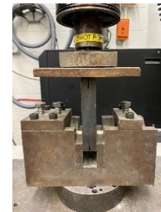
Transverse shear test setup
