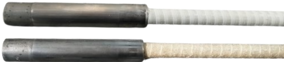
Coupler and GFRP rebar after swaging
