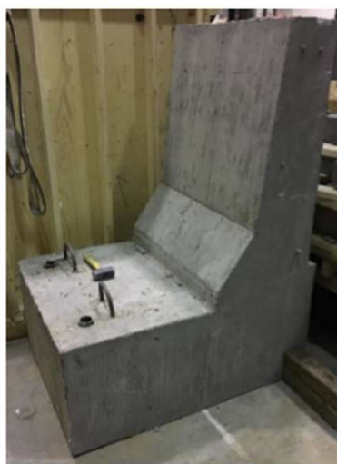
e) Barrier with rigid base
