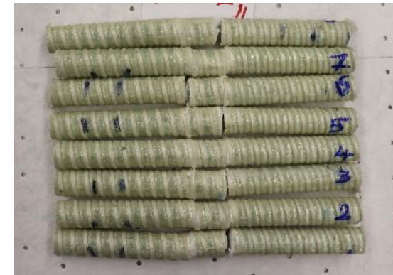
Typical shear failure
