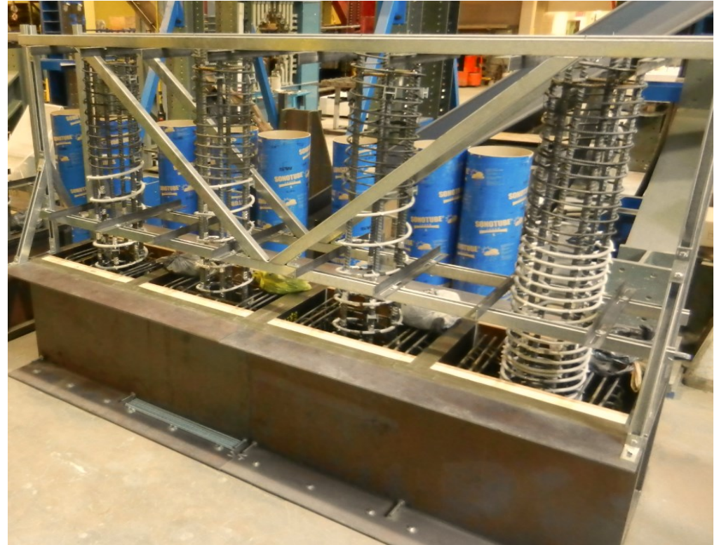
3. Cages Assembled in formwork
