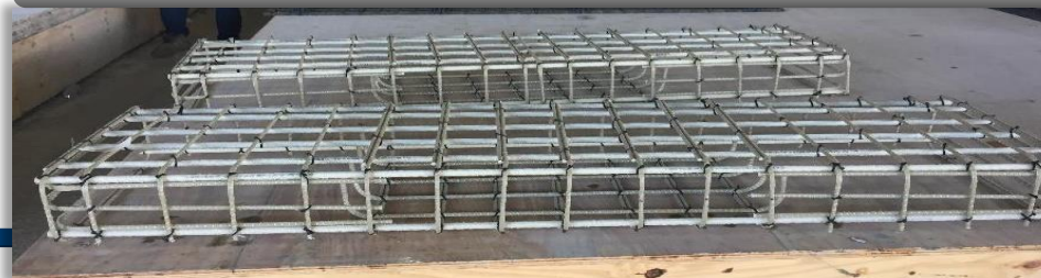
iDock pile bent caps GFRP rebar cages, Coreslab (2018)
