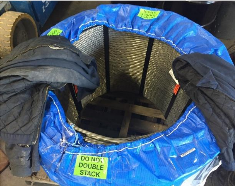
FIGURE: FDOT research facility coil of HSSS-alloy 2205, 0.6” dia. strand.
