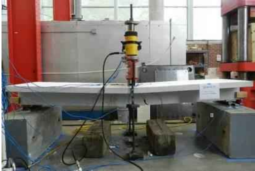
Figure 6.28: Failure of beam#8 after 12 months of exposure (Bottom Beam).
