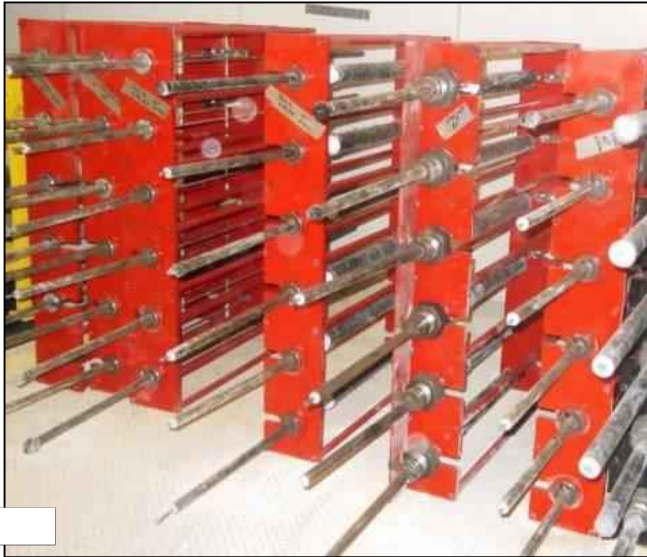
Figure 3.16: Sustained creep load frame during fixing the CFRP specimens with and without alkaline solution: (a) T=22^{\circ}\text{C} [72]; (b) T=60^{\circ}\text{C} [140°C]
