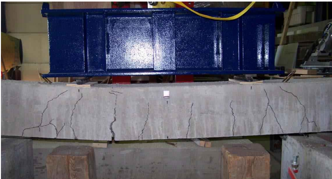
Figure 4.55: Crack pattern of the control beam specimens
