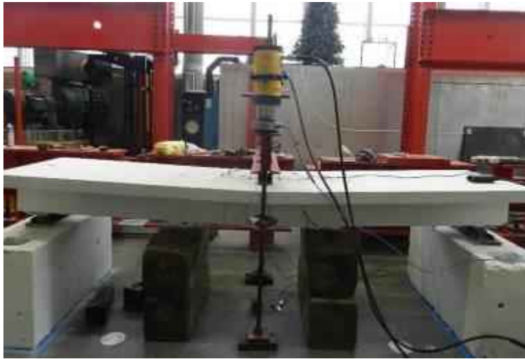
Figure 6.15: Failure of control beam#1
