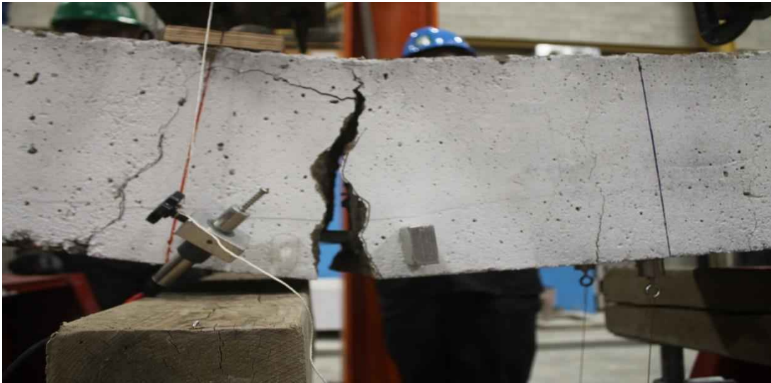
Figure 4.52: Flexural tension failure mode observed in all of the control and conditioned specimens
