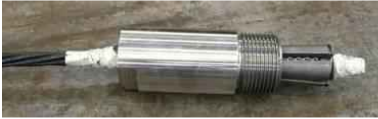
(i) Sleeve with wedges pressed inside it
