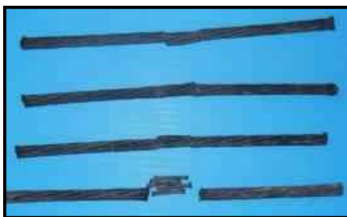
Figure 3.32: Typical shear failure of CFRP specimens
