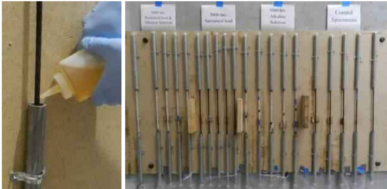
Figure 3.9: Preparation and curing of anchorages at NCSU
