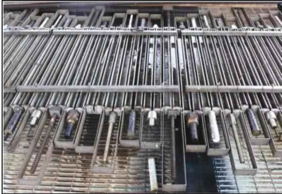
Figure 2.18: FRP cables pre-stressed in SUS flames (Sasaki and Nishizaki 2015)
