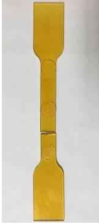
Figure 5.13: Typical failure mode of epoxy resin coupons.
