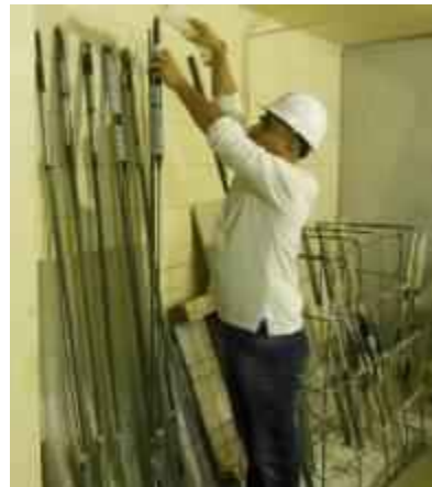
Figure 3.5: Anchorage preparation at Sherbrooke University
