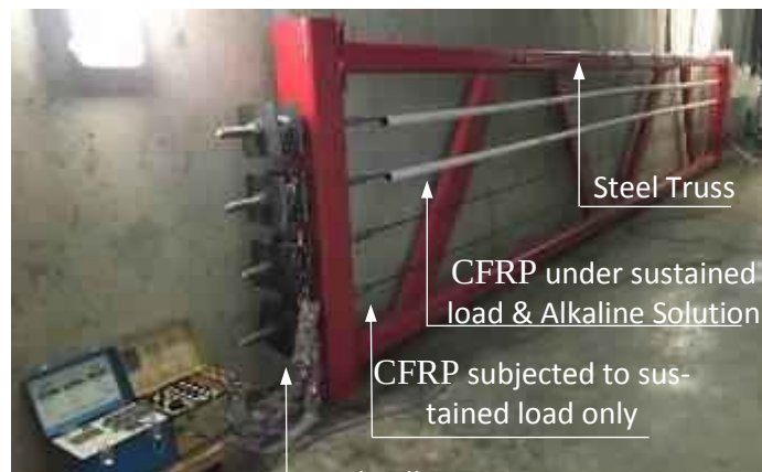
Figure 3.20: Steel truss with 4 tensioned CFRP tendons
