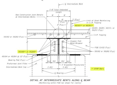
Top Innovations Employed: Utilization of GFRP bars and adoption of link-slabs to provide lateral load distribution and eliminate intermediate support expansion joints, without significantly restricting superstructure rotation at the support that could otherwise create secondary forces and cracking stresses.
