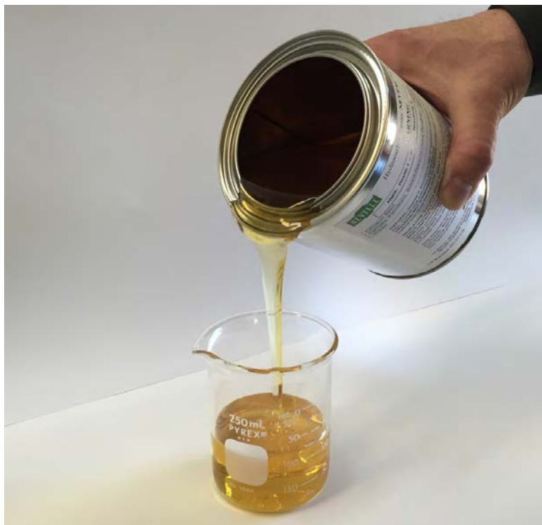
Figure 1.7: Thermoset resin used in FRP
