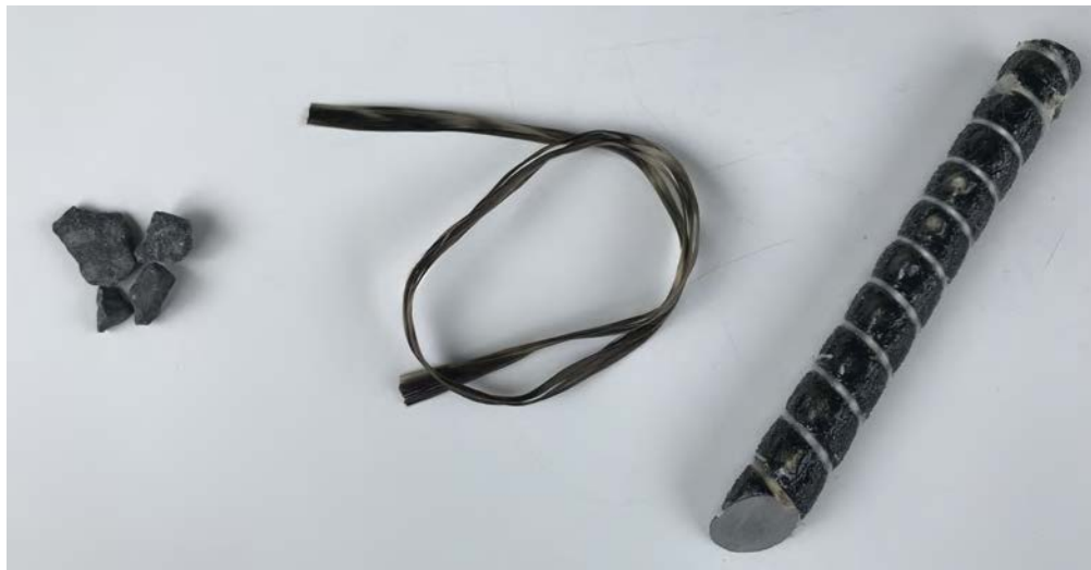
Figure 1.1: Basalt rock, fiber, and rebar
