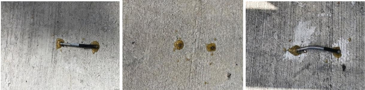
Figure 2.7: Vandalized surface mounted crackmeters
