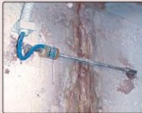
• Model 4420 Crackmeter installation.
