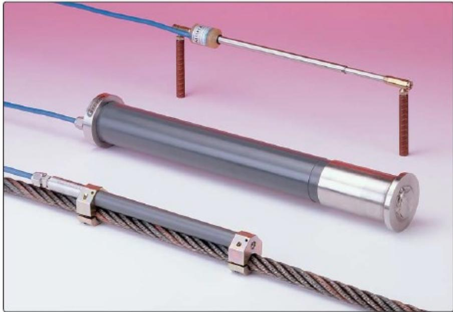
• Model 4410 Strandmeter (front), Model 4400 Embedment Jointmeter (center) and Model 4420 Crackmeter (rear).
