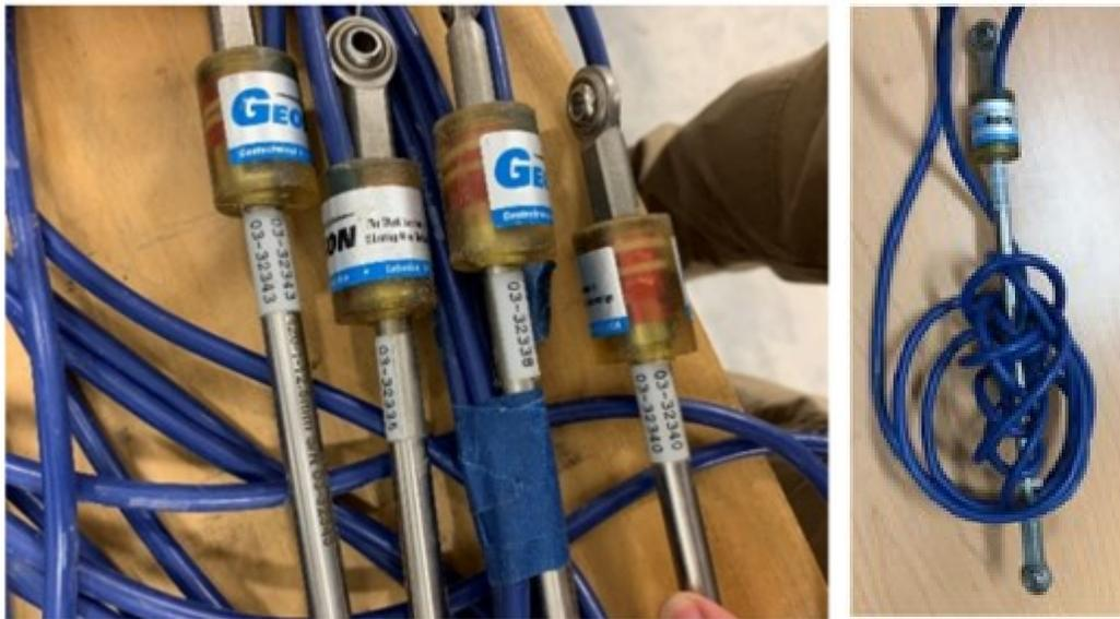
Figure 2.9: External displacement transducers
