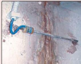
• Model 4420 Crackmeter installation.
