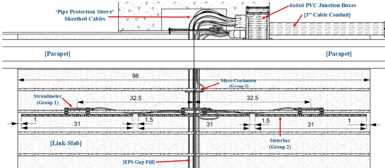
Figure 35, Drawing, Top View Detail of Link-Slab (Southwest Side)
