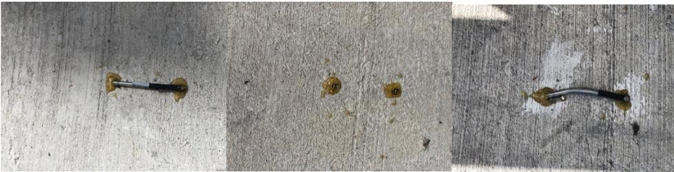
Figure 16. Vandalized sensors (crackmeters)
