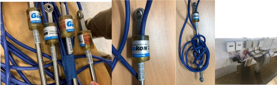
Figure 15. Installed Sensors (surface mounted)
