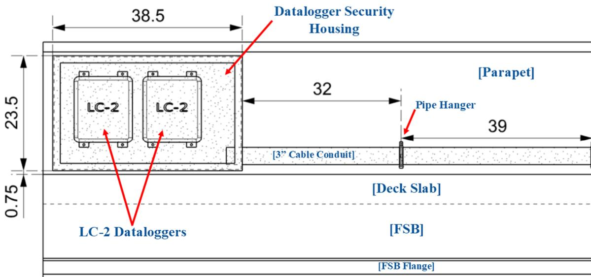
*Figure 34, Drawing, Bridge Side View No.3 (Detail of Data Acquisition)*
