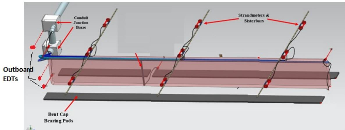
*Figure 27, Exposed View of Cable Routing (EPS is Translucent)*
