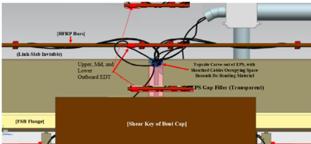
**Figure 9, Detail of Embedded Sensor Routing, Side View**
