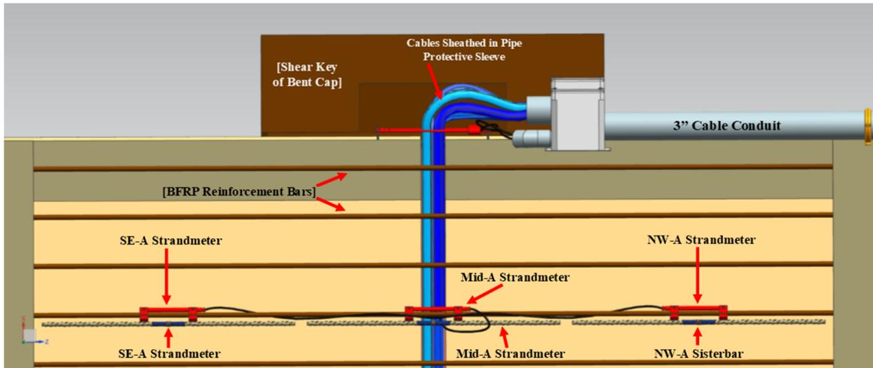
*Figure 2, Detail of Embedded Sensors, Top View*
