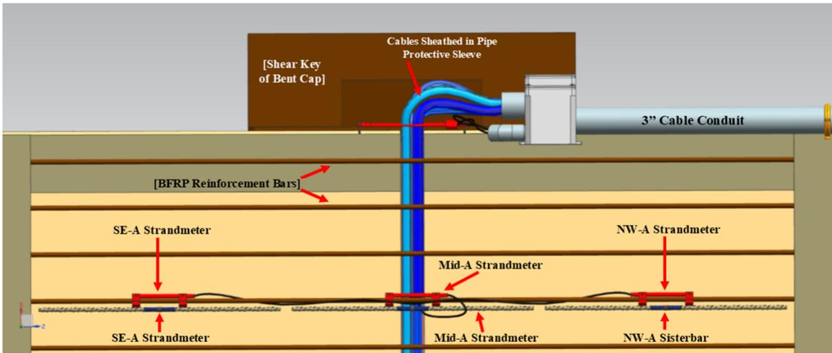
*Figure 25, Detail Link-Slab, Top View*
