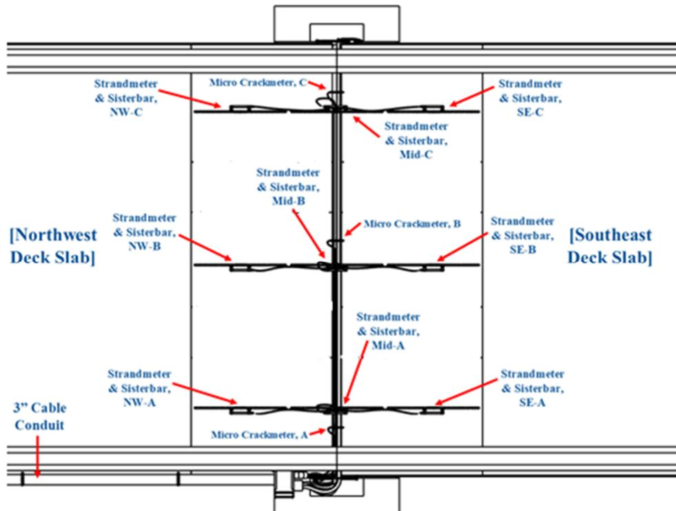
*Figure 28, Drawing, Labels of Embedded Array and Micro Crackmeters*
