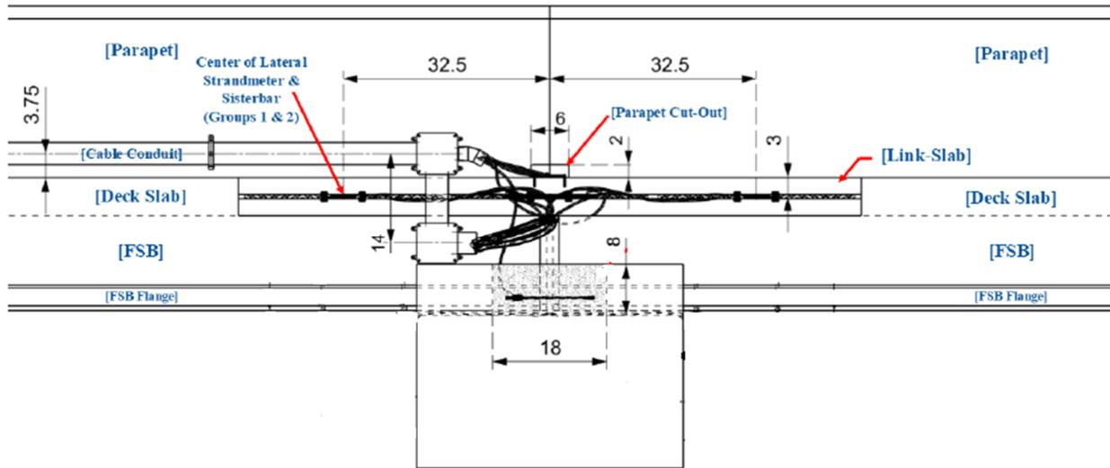
*Figure 33, Drawing, Bridge Side View No.2 (Detail of Link-Slab)*
