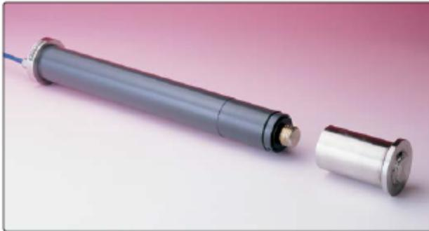
• Model 4400 Embedment Jointmeter shown with socket removed.
