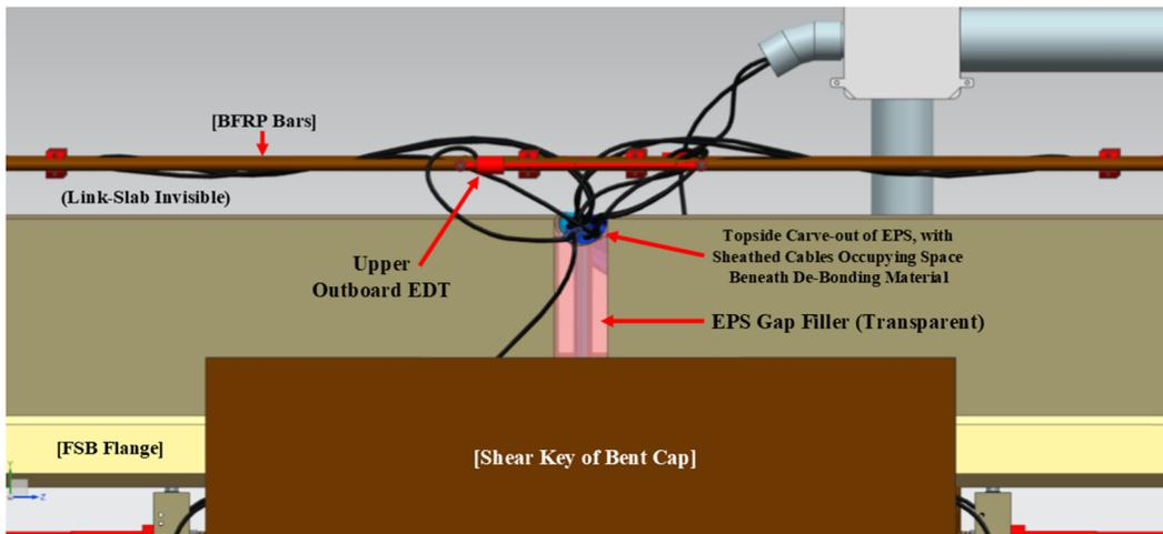
*Figure 26, Side View of Exposed Embedded Sensors and BFRP rebars*
