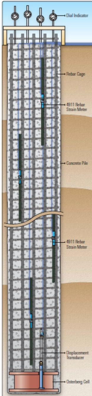
• Installation of the Model 4911 in an Osterberg Cell pile test. (For more information regarding Osterberg Cell pile testing, please contact Loadtest, Inc. — [www.loadtest.com](http://www.loadtest.com)).
