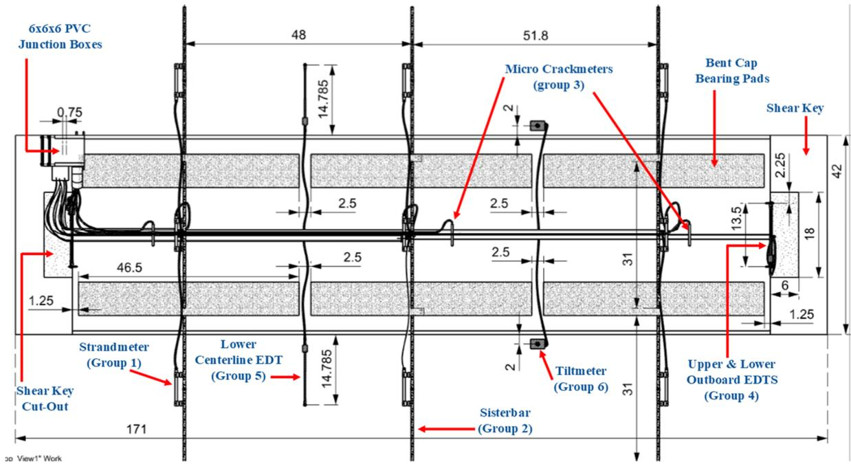
Figure 90, Drawing, Bent Cap Top View (Slabs, Beams, and Parapets not Shown)
