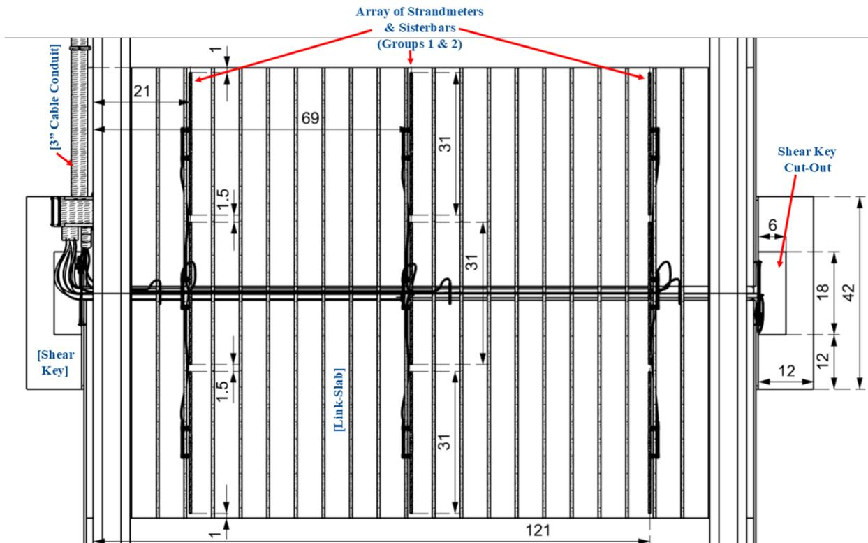
Figure 36, Drawing, Top View of Whole Link-Slab
