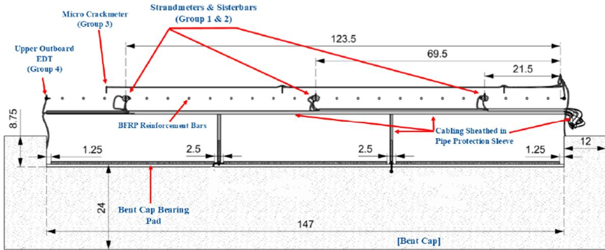
Figure 29, Drawing, Bent Cap End View (Slabs, Beams, and Parapets not Shown)
