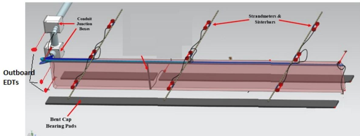
**Figure 7, Cable Routes Through EPS**
