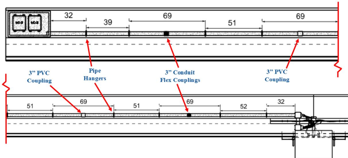
Figure 32, Drawing, Bridge Side View No.1 (Wide)
