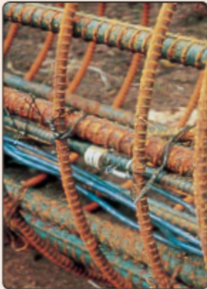
• Close-up of Model 4911 shown as installed in concrete pile reinforcing cage.
