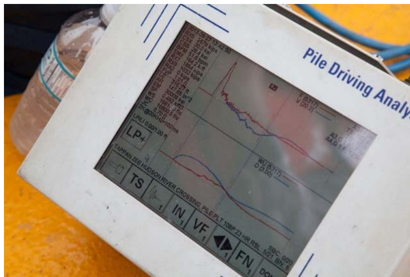
Figure 1.4: Pile Driving Analyzer (PDA).
