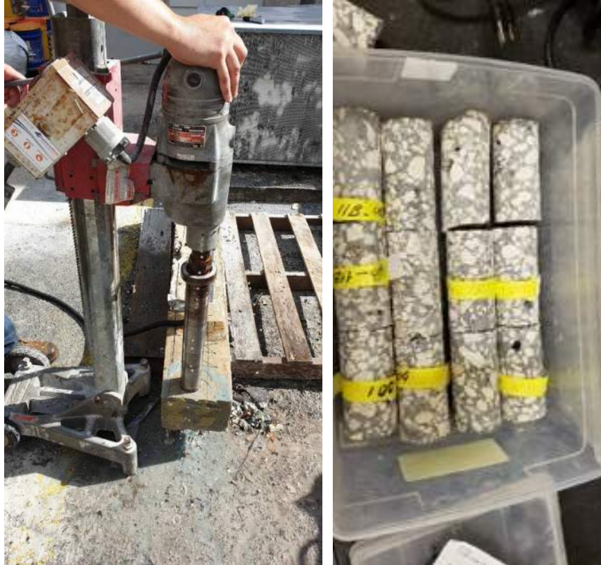
Figure 4 – Coring activities on test blocks
