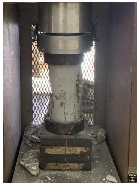
Representative Failure Mode:
