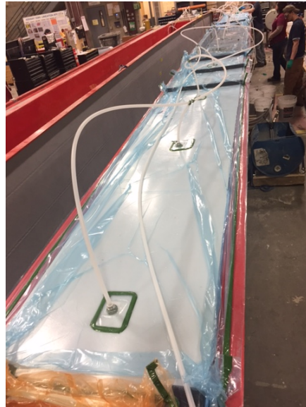
Figure 118: HCB resin infusion setup
