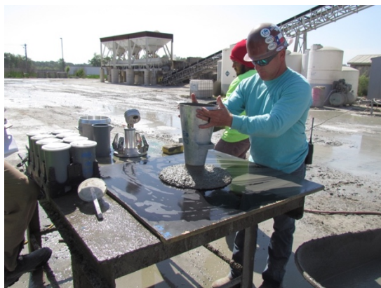
Figure 164: Testing for SCC spread
