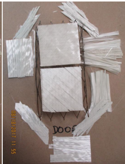
Figure 143: FDOT samples 4 th layer 102 oz removed (FDOT)
