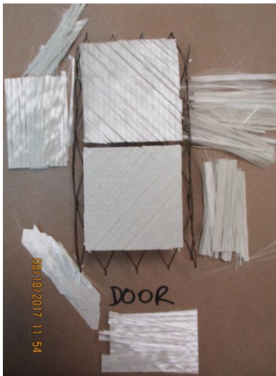
Figure 142: FDOT samples 3 rd layer 102 oz removed (FDOT)
