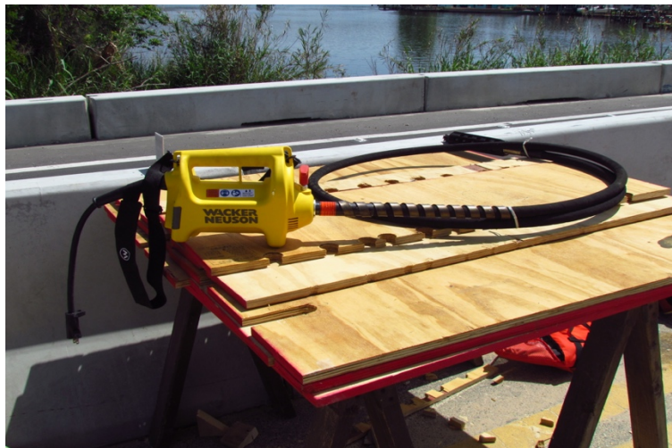
Figure 99: Rubber tip vibrator
