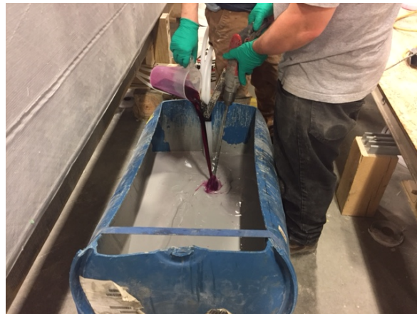
Figure 119: Mixing of resin with hardener during resin infusion
