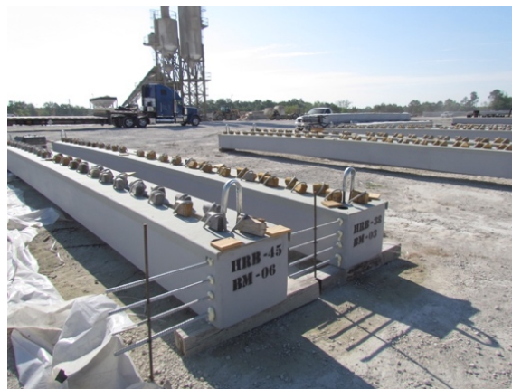
Figure 162: HC beams supported by 4x4
