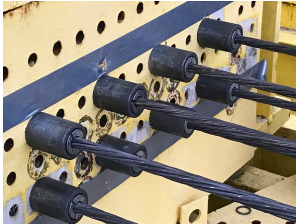
Figure 64: Open grips on steel strands
