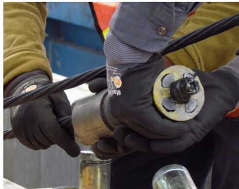
Figure 25: Wedge seating CFCC strand
