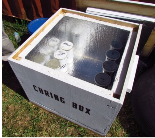
Figure 97: Curing box with concrete cylinders
