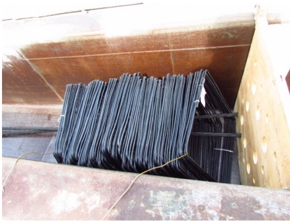
Figure 22: Secured CFCC spirals
