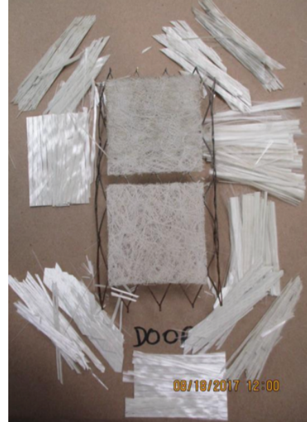
Figure 145: FDOT samples 2 nd layer 24 oz removed (FDOT)
