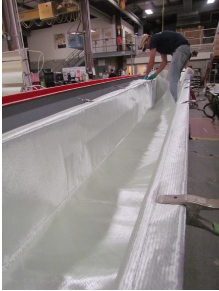
Figure 111: Blue release film and fiberglass layers
