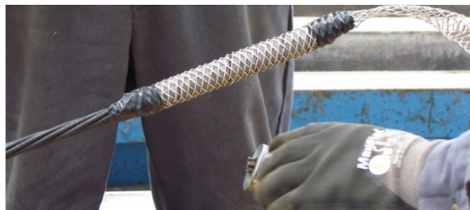
Figure 24: Stainless steel mesh on CFCC strand
