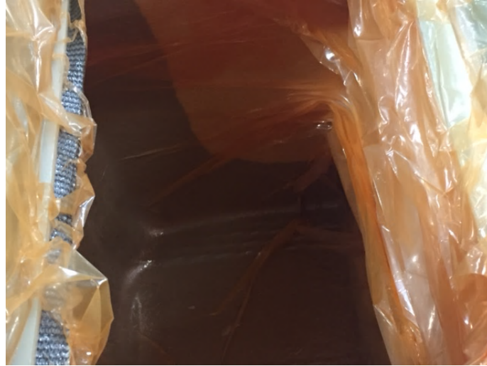
Figure 120: Resin flow in HCB chimney
