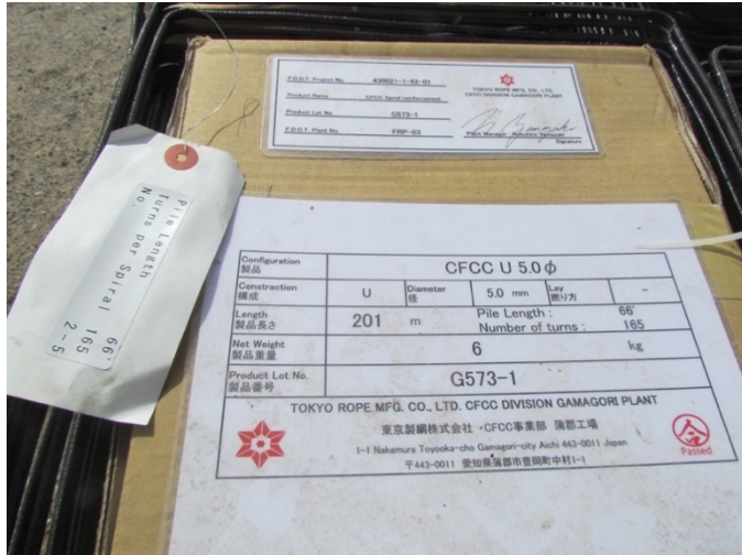
Figure 20: Label on CFCC spirals
