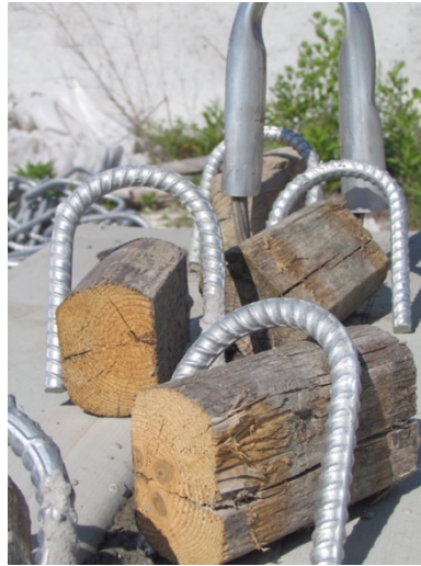
Figure 163: Uneven shear connectors
