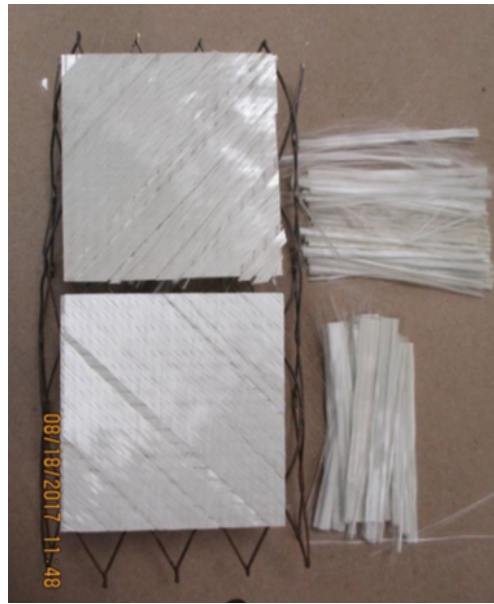
Figure 140: FDOT samples 1 st 102 oz layer removed (FDOT)
