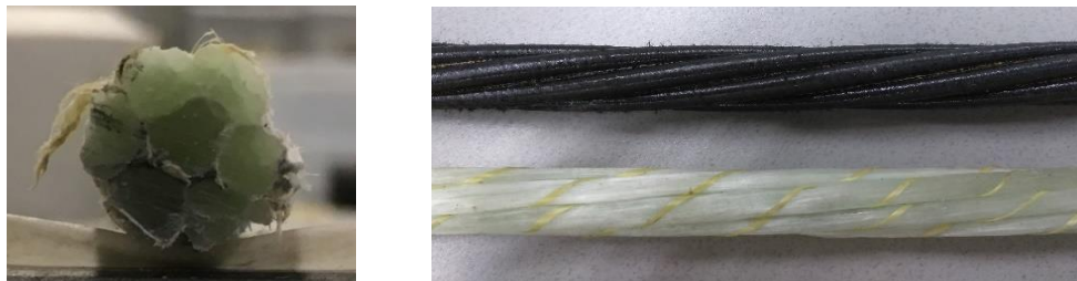
(a) GFRP strand prototype cross section; (b) compared to a CFRP alternative.
