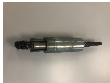
Wedges and couplers of CFRP and Standard prestressing steel
