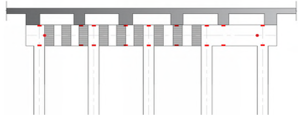
Strain gage locations for bent caps 37
