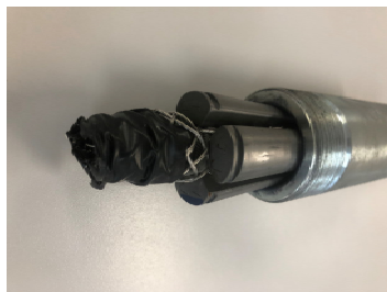
Wedges and couplers of CFRP and Standard prestressing steel
