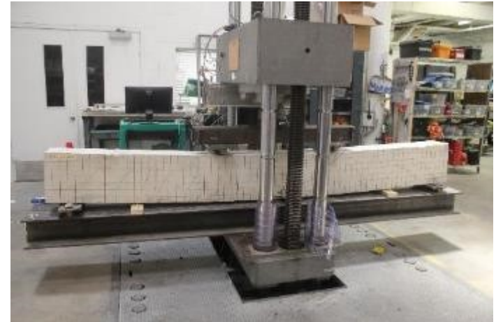
Testing of GFRP-RC beam using four-point setup
