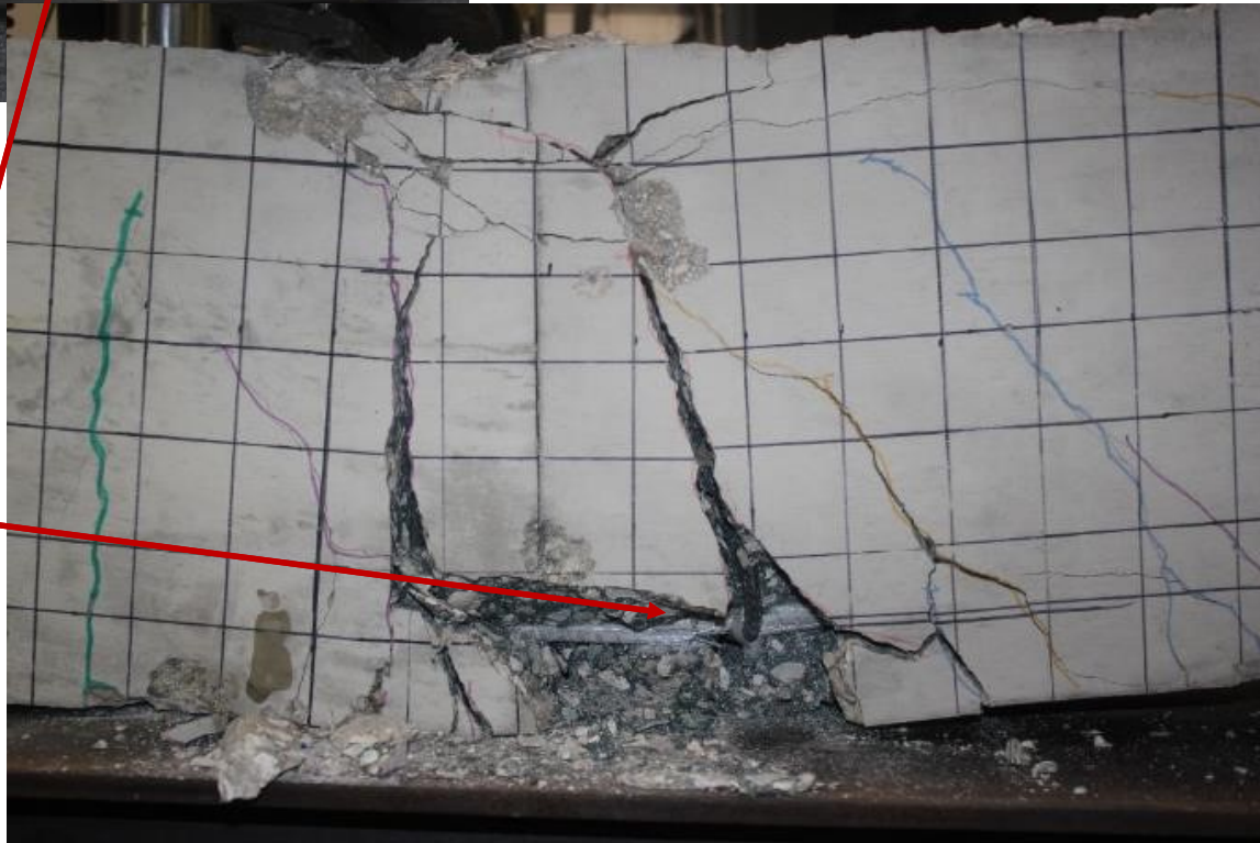
FRP Rupture Failure in GFRP Reinforced Beam
