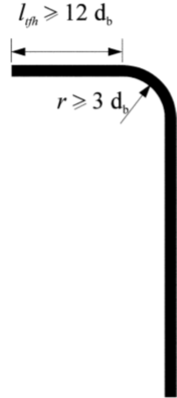
Minimum radius and tail length of a stirrup bend
