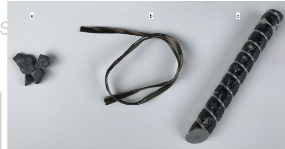
Figure 2.1: (a) Basalt rock, (b) Fiber, and (c) Rebar
