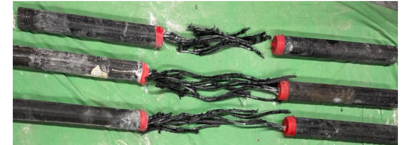
Charts and Photos: Tensile strength development and failure mode after 7 years of embedment in seawater concrete for (a) BFRP, (b) GFRP, and (c) CFRP.
