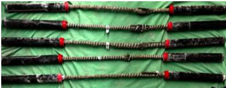
Charts and Photos: Tensile strength development and failure mode after 7 years of embedment in seawater concrete for (a) BFRP, (b) GFRP, and (c) CFRP.
