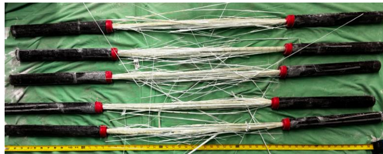
Charts and Photos: Tensile strength development and failure mode after 7 years of embedment in seawater concrete for (a) BFRP, (b) GFRP, and (c) CFRP.
