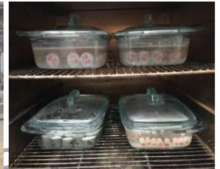
Comparative durability of cement-embedded and bare GFRP bars
