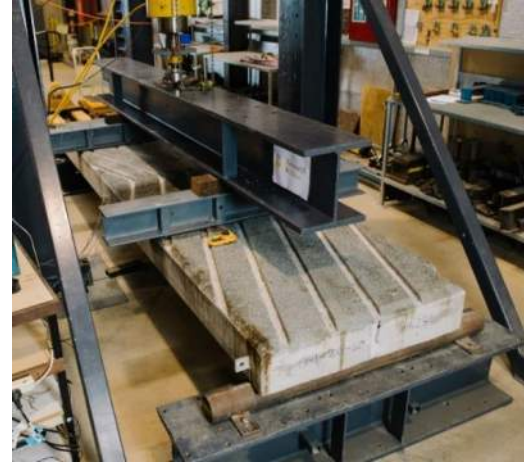
Test set-up for boat ramp planks
